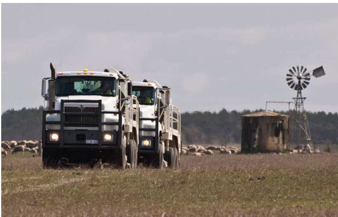
Vibrator trucks in action during 3D seismic recording at Windermere, Otway Basin
