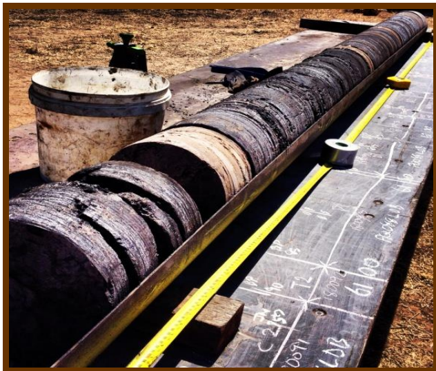
Figure 2 : Large diameter core extracted at Washpool
