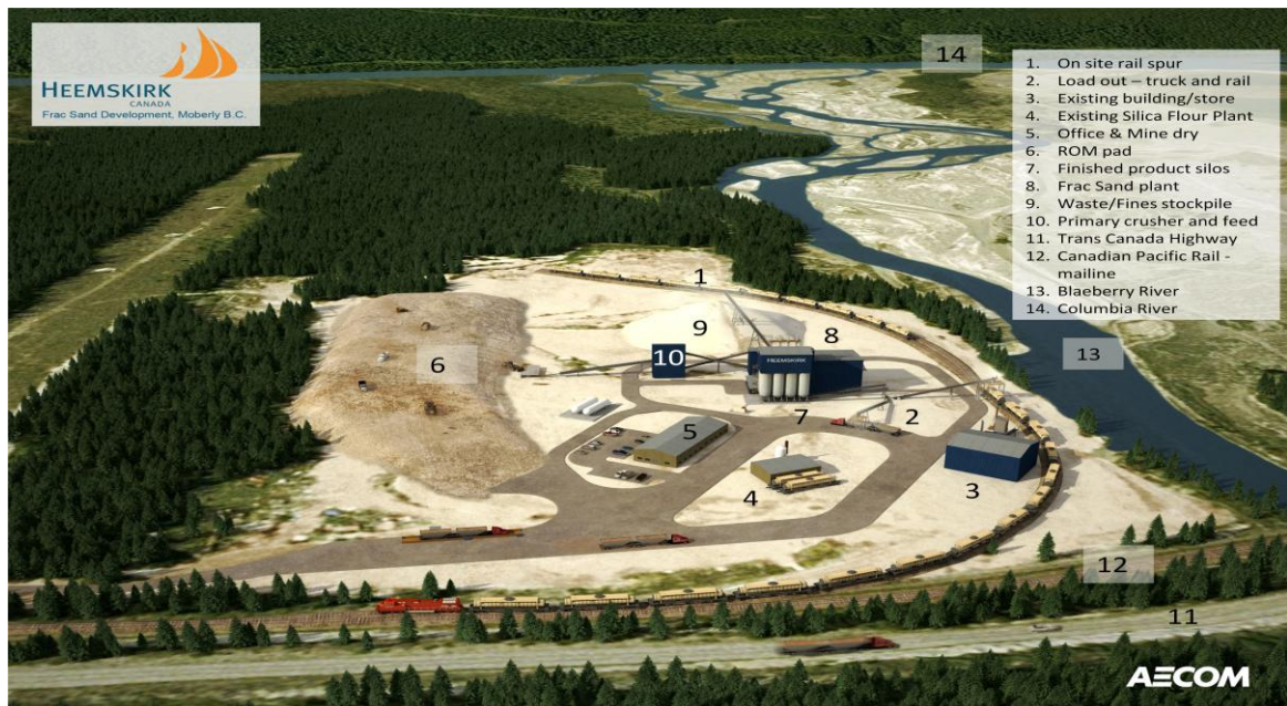
Figure 5: Layout of proposed plant at existing Moberly Plant Site (no land clearing required)
