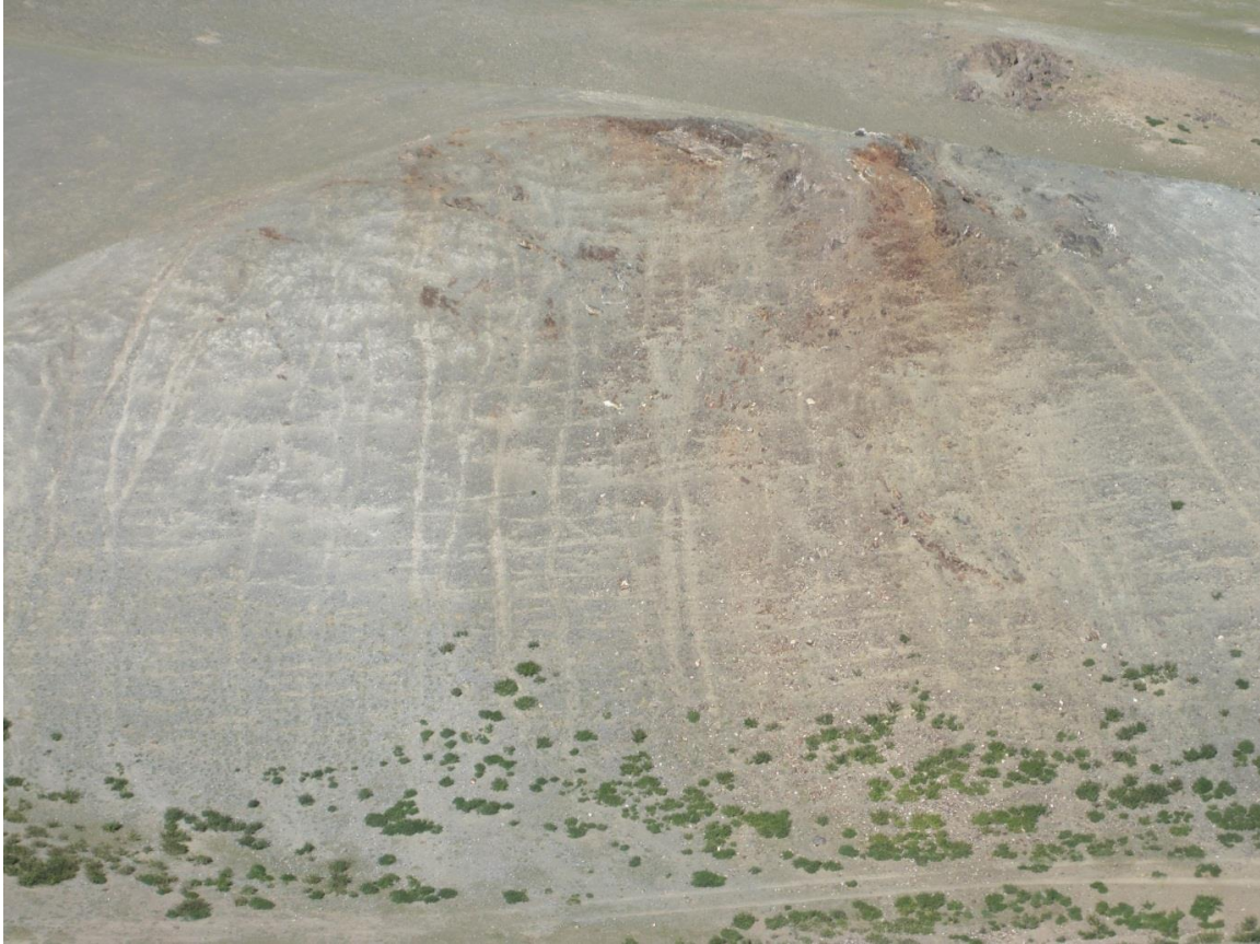
Figure 7 Quartz-gossan-malachite-azurite outcrop at Mushroom East with rock chip grades up to 5.56% Cu and 0.44 g/t Au
