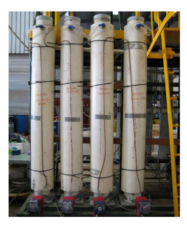
Successful 2 metre bioleach high columns which gave up to 85% recovery of the uranium
