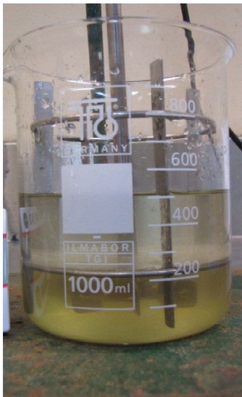
Figure 4. Solvent extraction phase disengagement testwork showing that the pregnant leach solution produced does not form third phases or 'cruds'. Phase disengagement time was fast regardless of continuity.
