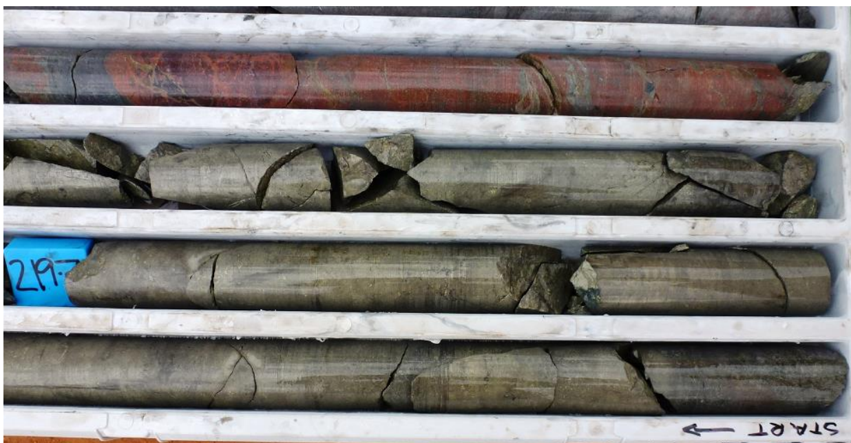
Figure 5. Hole EEDD012 – portion of massive sulphide interval from 217.5 metres to 221.5 metres
