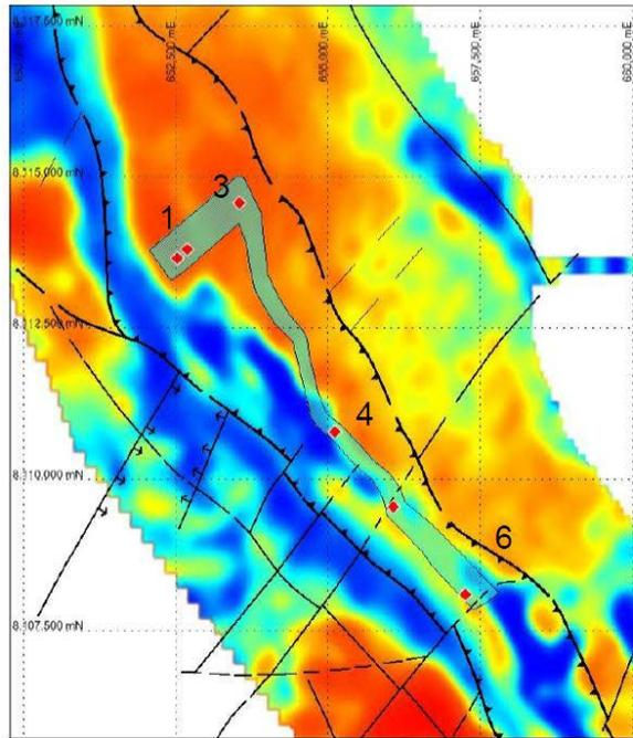
**Figure 2.** Geology interpretation and proposed drillholes superimposed over AEM image 150 – 200m conductivity depth slice .
