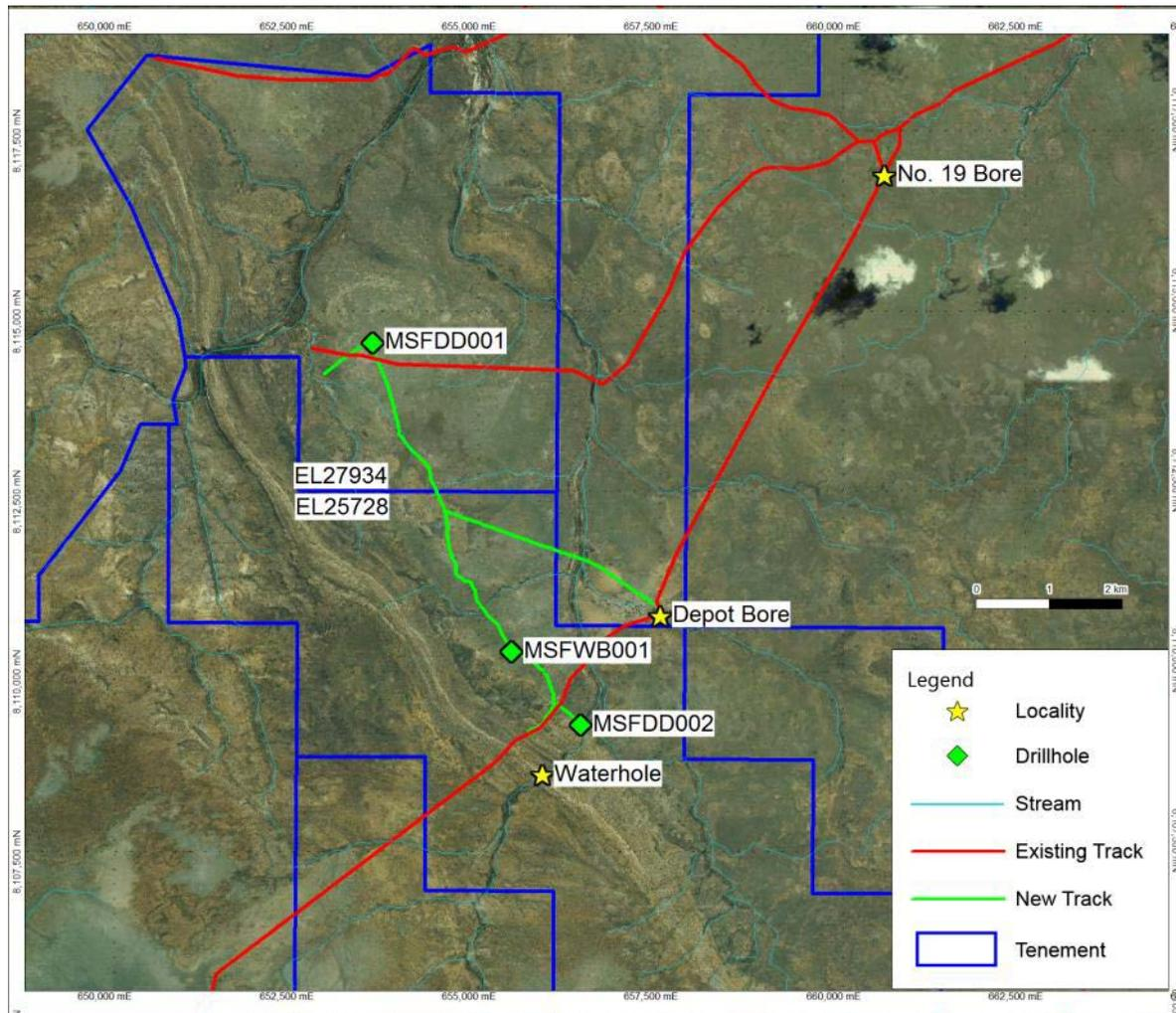
**Figure 3.** Project drillhole collar locations and access tracks with satellite imagery background. All coordinates in MGA zone 52 GDA94 and all elevation in AHD. All azimuth measurements are magnetic - magnetic declination at time of survey measurements was 3.5°.
