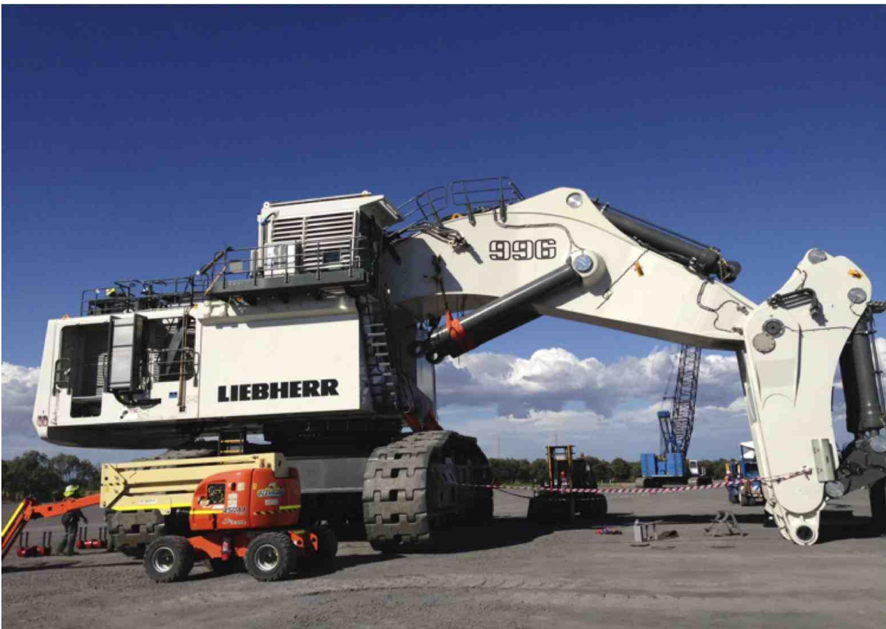
Figure 2 - Liebherr 996 Excavator being constructed at Baralaba North
