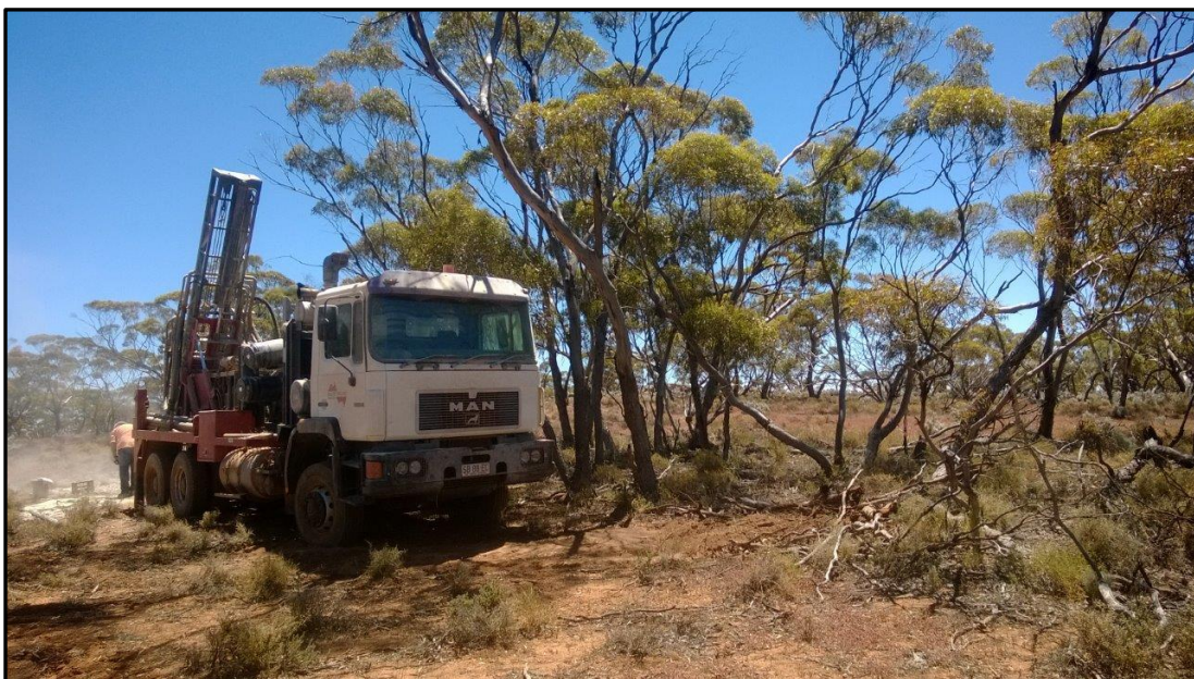
Figure 2: Photo of aircore drilling at Frakes prospect, Menninnie Dam.
