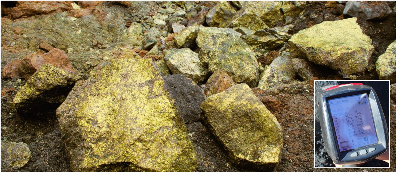
Figure 02: Massive primary copper ore chalcopyrite (yellow - chalcopyrite contains 34.6% copper) and clay-rich chalcocite (black/brown/grey - chalcocite contains 79.8% copper). The chalcopyrite is associated with chalcocite, resulting in very high copper grades. XRF result shows reading of chalcocite-rich chalcopyrite.
