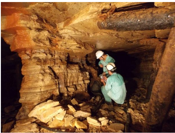
Figure 5. Bulk sampling at the Cuca winze, approximately 400m north of the planned exploration decline.
