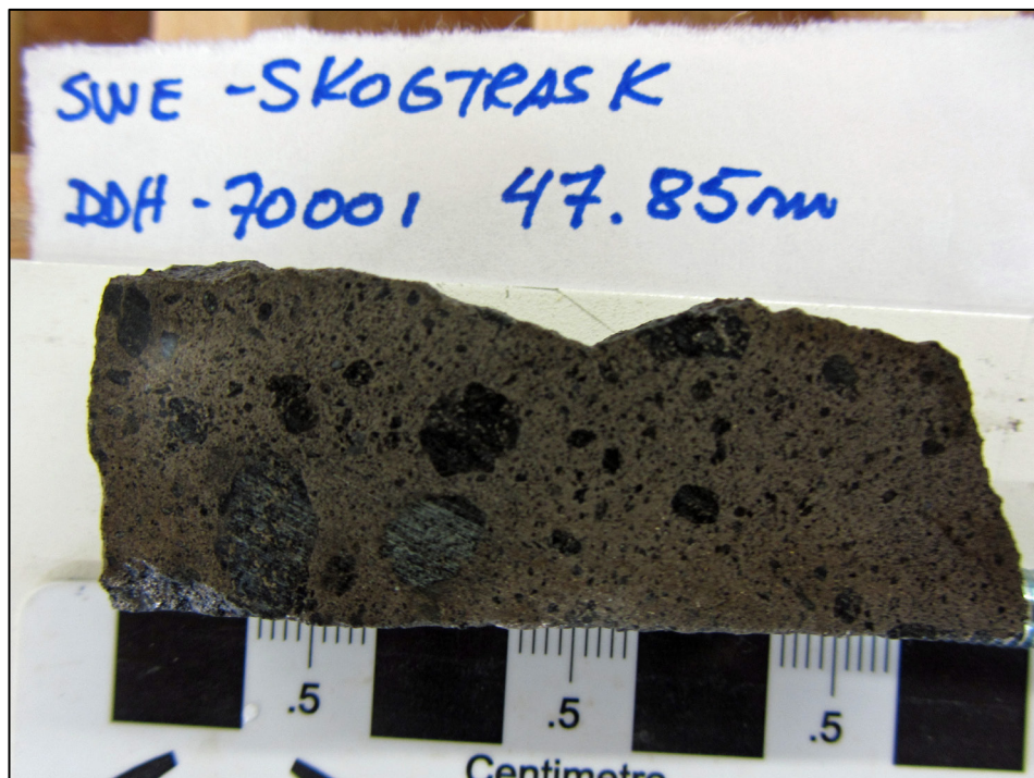
Figure 6. Photograph of quarter core with semi-massive Ni-Cu sulphides grading 1.1% Ni and 0.2% Cu, drilled by the Swedish Geological Survey and kept in their Mala Core Farm, Sweden (hole DDH 7001, 47.8 m down hole depth)
