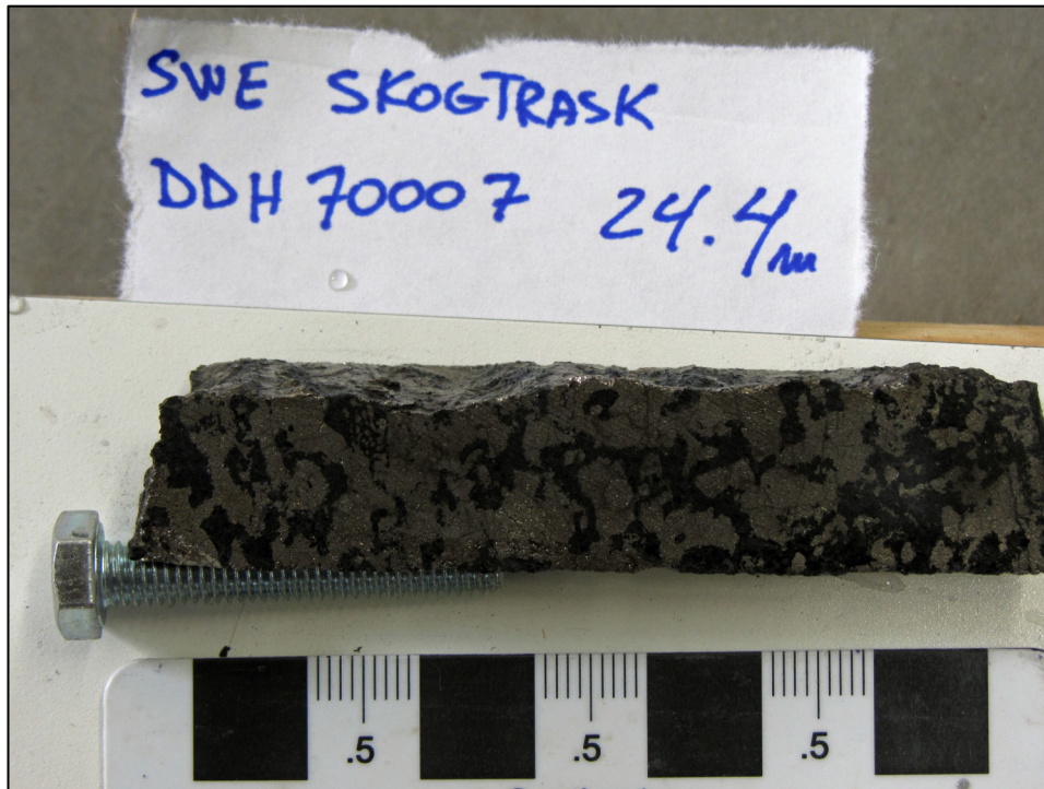
Figure 5. Photograph of quarter core with semi-massive Ni-Cu sulphides grading 0.9% Ni and 0.4% Cu, drilled by the Swedish Geological Survey and kept in their Mala Core Farm, Sweden (hole DDH 7007, 24.4m down hole depth)
