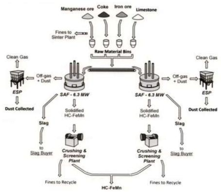
Process flow diagram for high carbon ferro manganese smelter
