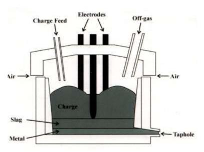
Schematic Cross-section of Submerged Arc Furnace
