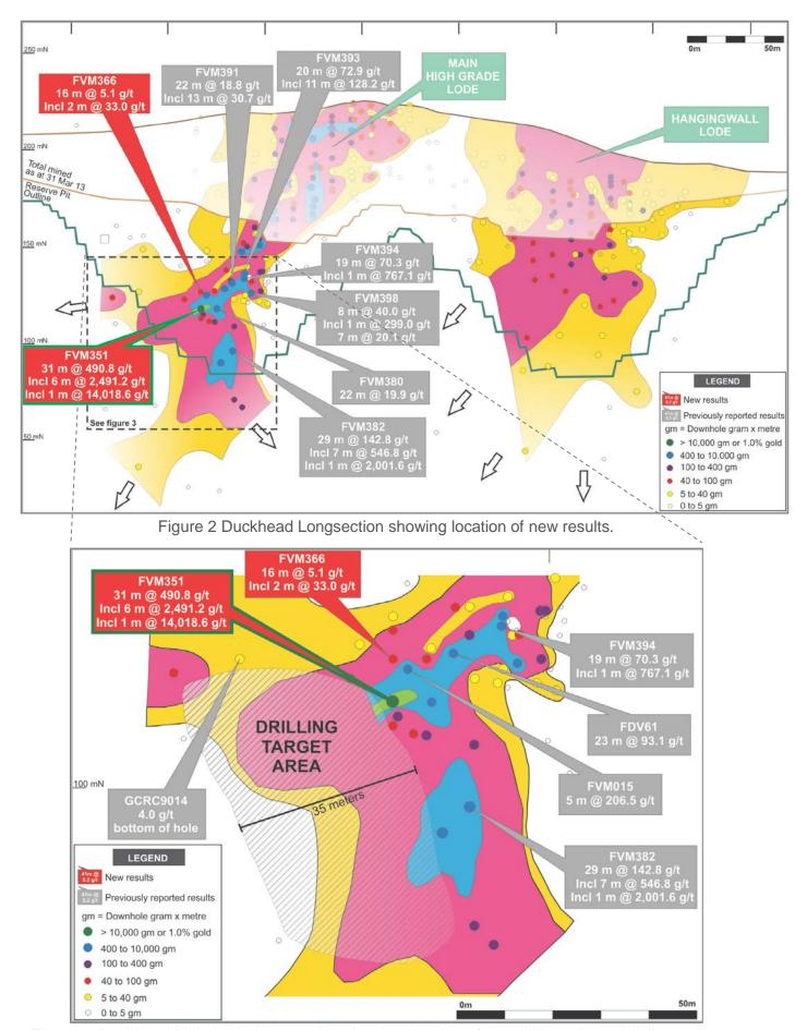
Figure 3. Duckhead Main Lode Longsection showing location of new drill results and drill target area.
