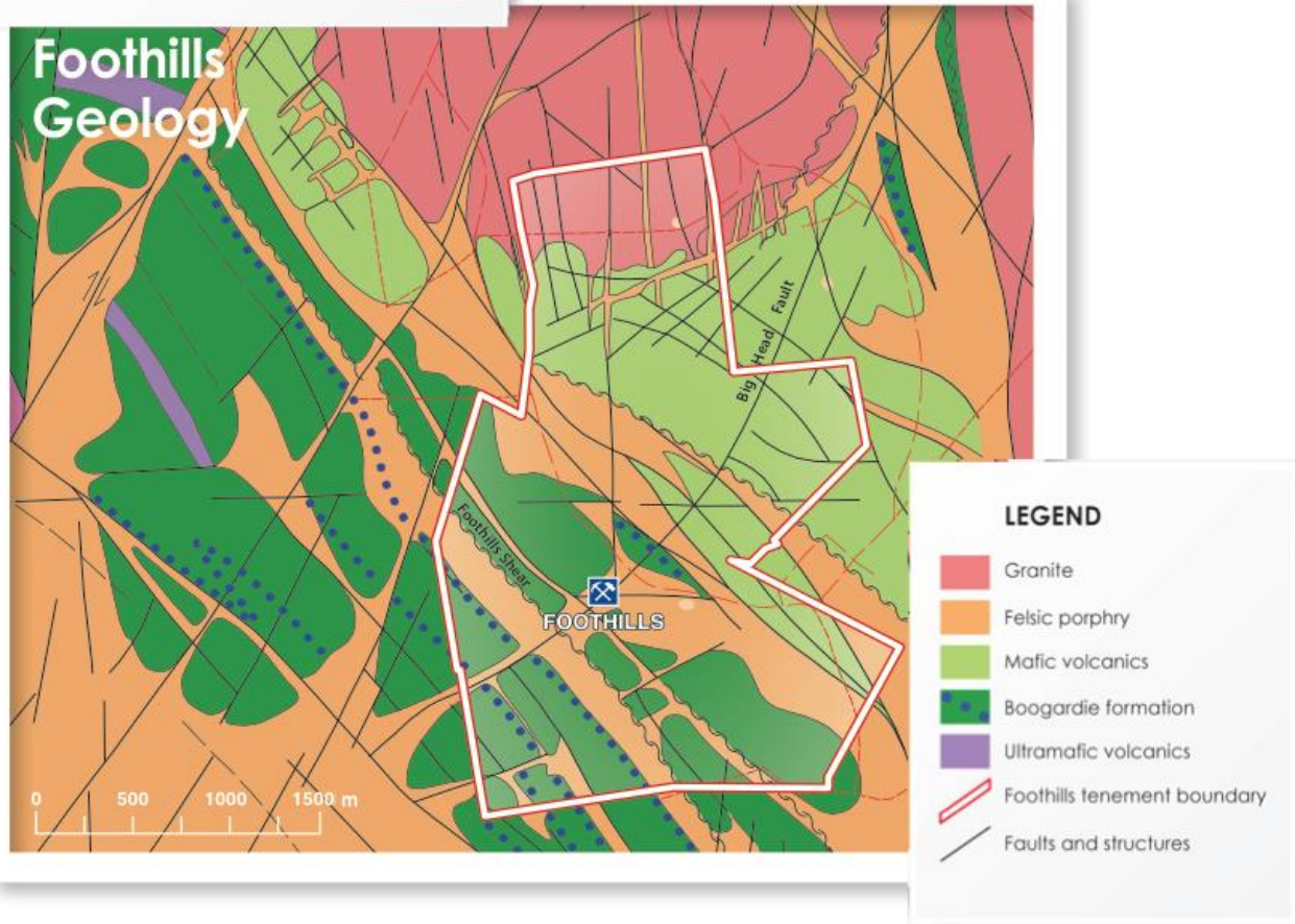
Figure 2: Simplified geology of the Foothills prospect. The approximate positions of the Big Head Fault and Foothills Shear as shown are based on broad-spaced airborne geophysical data. As these geological structures are thought to play a role in controlling primary gold and copper mineralisation at Foothills, it is important that Australian Mines accurately determine their location at depth.
