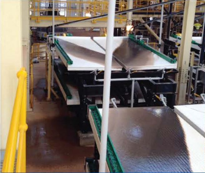
Shaking tables in the Wet Mill at the MSP
