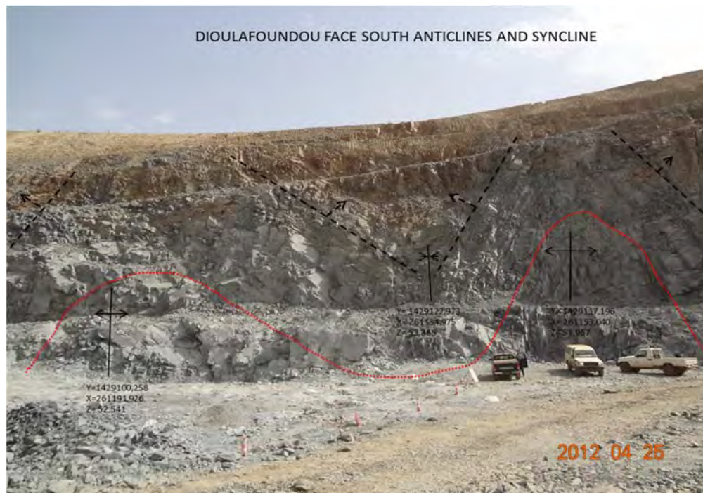
Figure 7-2 F1 Folding on South Wall of Dioulafoundou Pit (courtesy A. Maiga)
