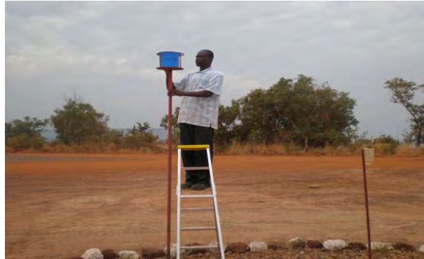
Figure 20-2 Technician Inspecting Dust Fall Out Monitor
