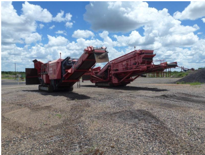
Figure 2: Terex J1175 Crusher and Terex Finlay 604 Supertrack Screen at Labusrus Plant Site
