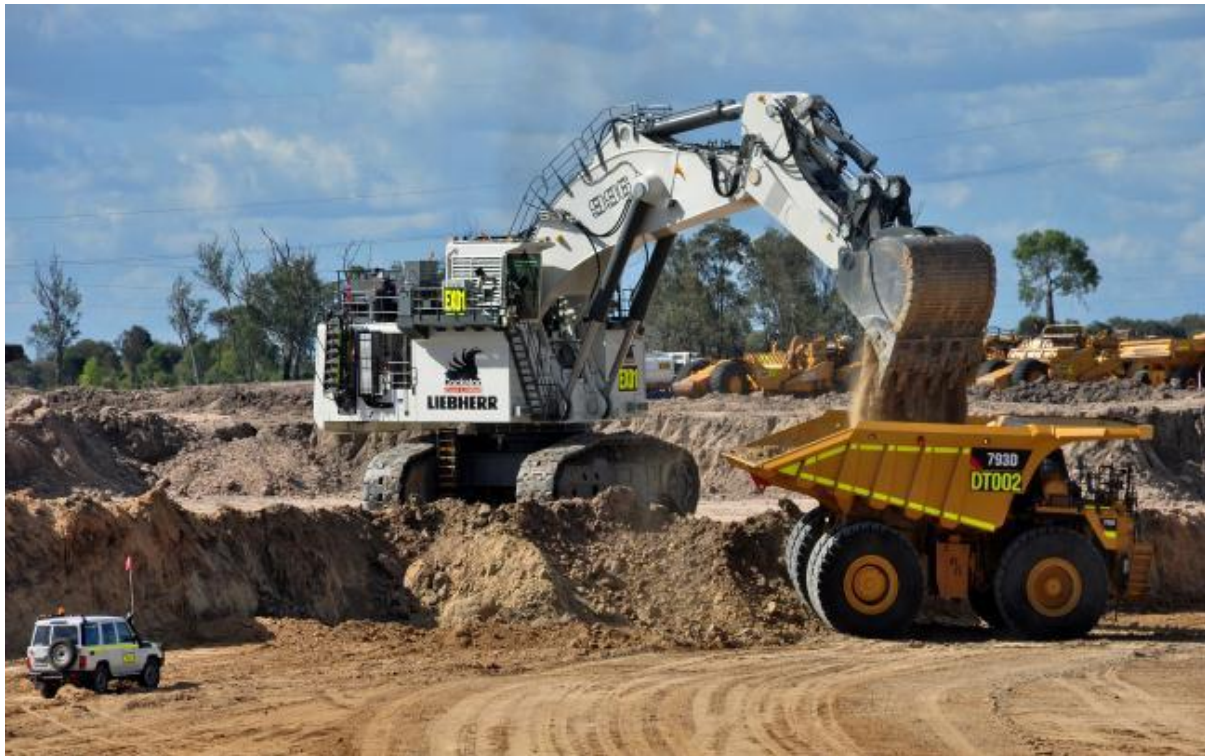
Figure 1 - Pre-stripping at Baralaba North (Liebherr 996 Excavator and Cat 793 Truck)
