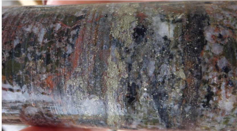
Figure 5: CRL001 – 66.65m drill depth, pyrite mineralisation associated with quartz and haematite veining and phyllic (quartz-sericite) alteration
