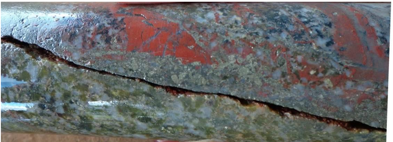
Figure 6: CRL001 – 75.5m drill depth, pyrite mineralisation associated with quartz and haematite veining offset by post-mineralisation structure for fault contact with strongly altered (propylitic) granodiorite host rock
