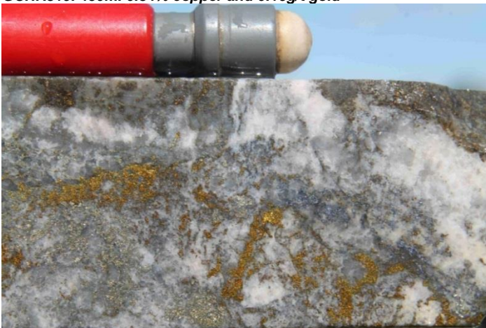
D vein dominated by quartz, chalcopyrite and molybdenite GCHR319, 456.3m. 1.98% copper, 0.24g/t gold, 13.1g/t silver and 1445ppm molybdenum.
