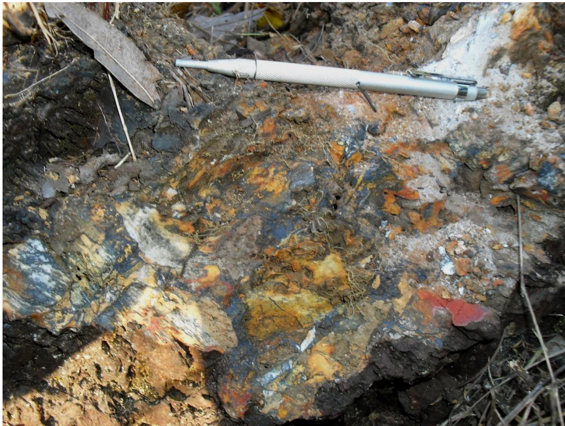
Figure 2. Sampling of this breccia outcrop showing hematite alteration returned grades of 4,234 g/t silver and 0.3% Copper.
