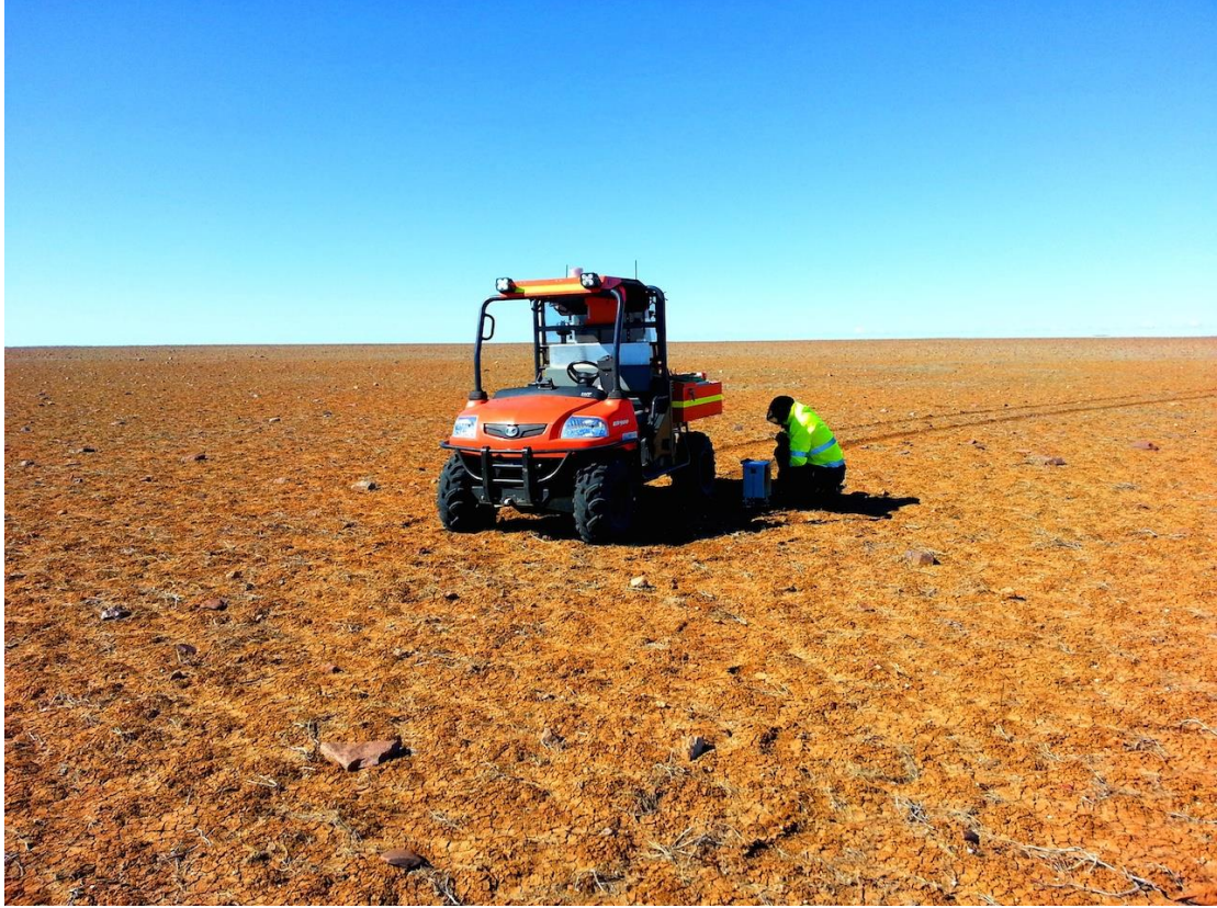
Figure 3: Daishat surveyor taking a gravity reading
