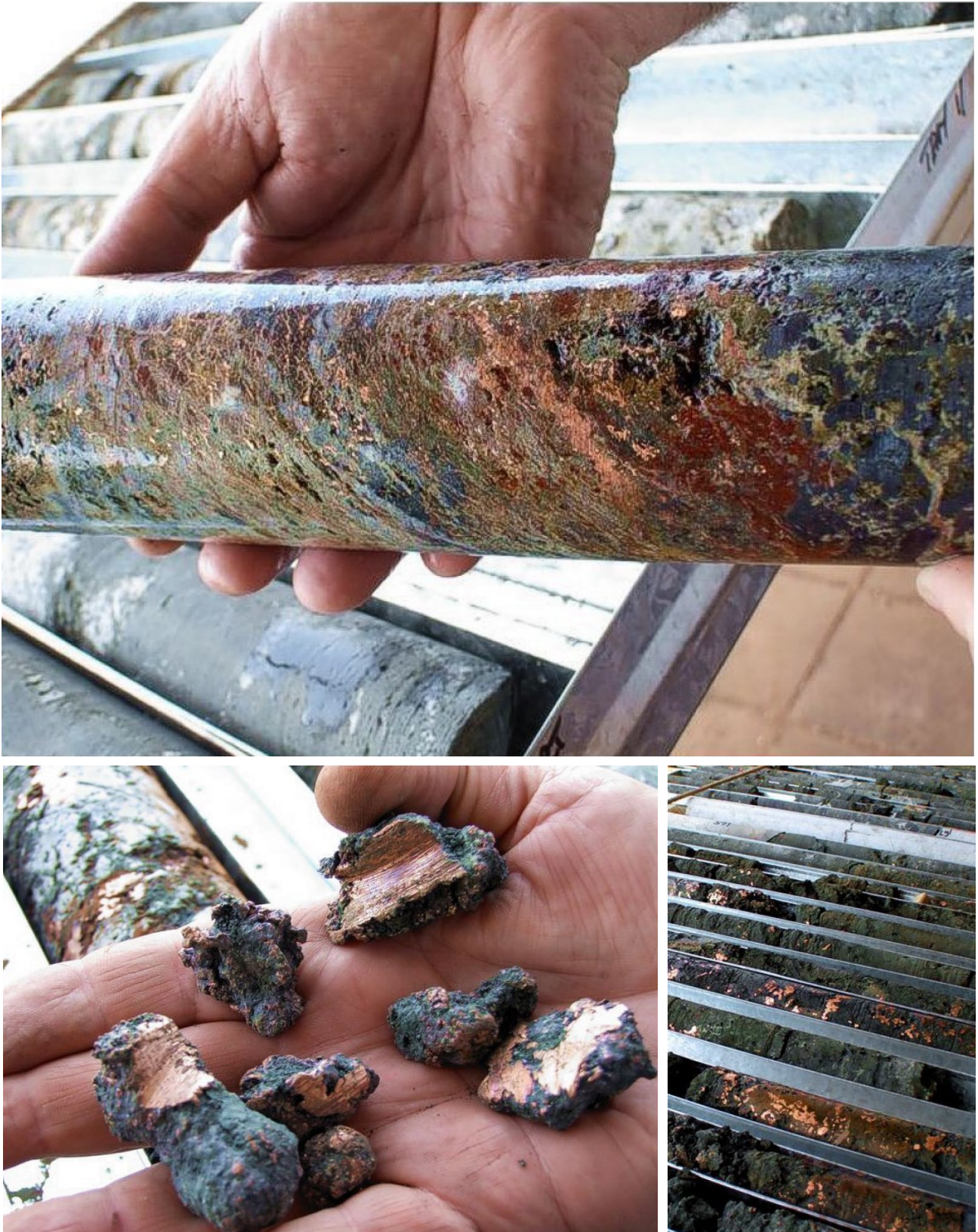
Figure 9: Examples of coarse native copper in metallurgical drill core from the Las Minerale Bonanza zone
