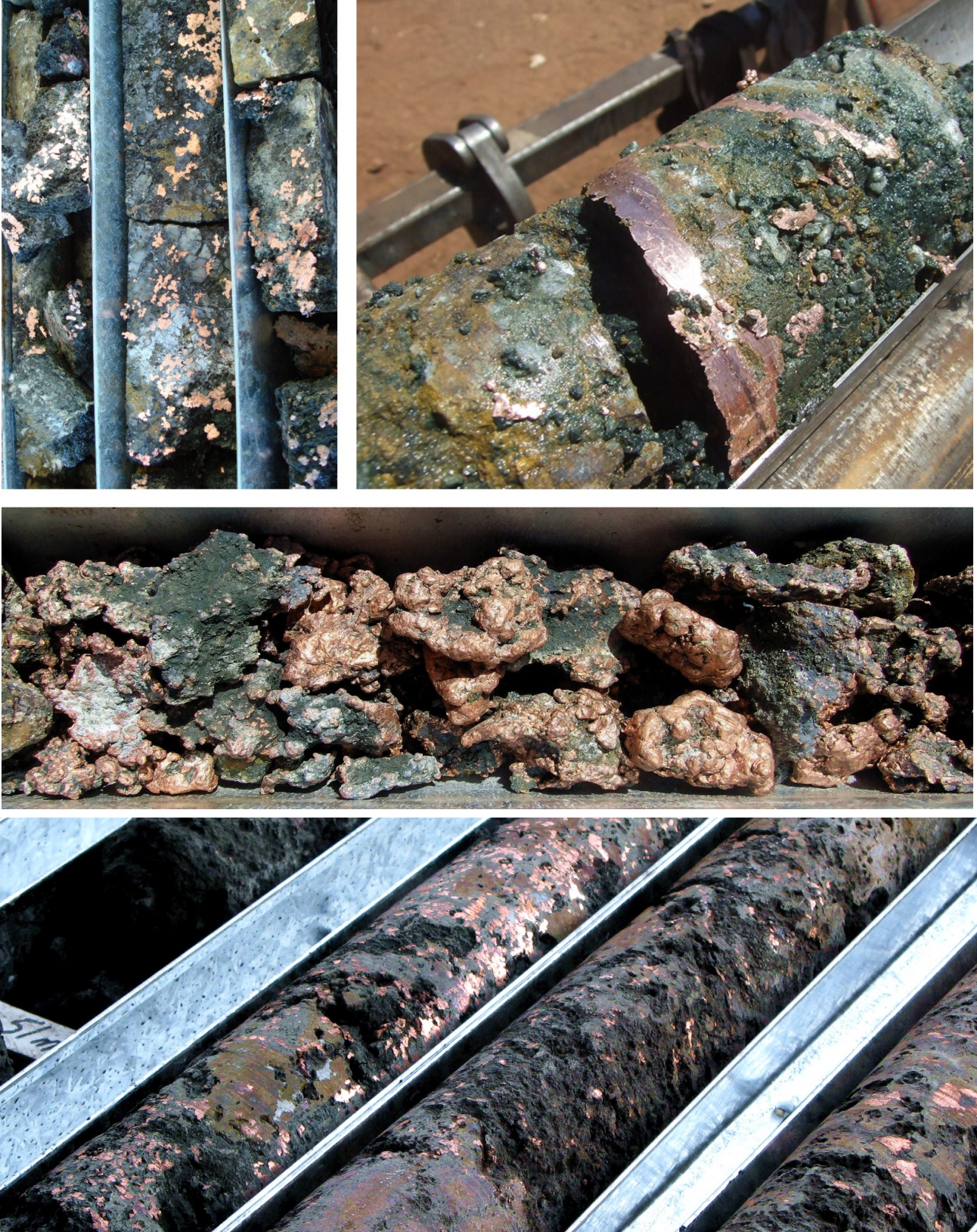
Figure 7: Examples of coarse native copper in metallurgical drilling in the Bonanza native copper ore zone.
