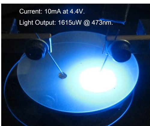
Figure 1: Demonstration of light emission at 473nm, with full width half maximum of 22nm, from a RPCVD p-GaN layer grown on a MOCVD partial structure.
