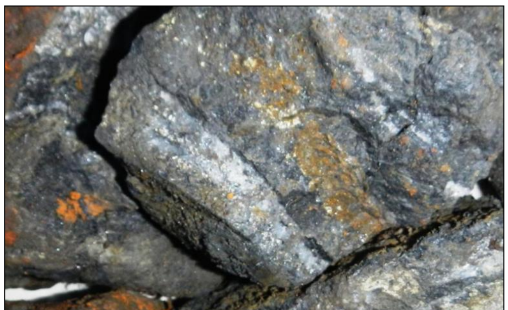
Photo 5. Strongly sulphidic (pyrite, arsenopyrite, sphalerite and galena) and silicified conformable gold mineralisation from the Lower Zone at J400, with 0.3m grading 197 g/t gold
