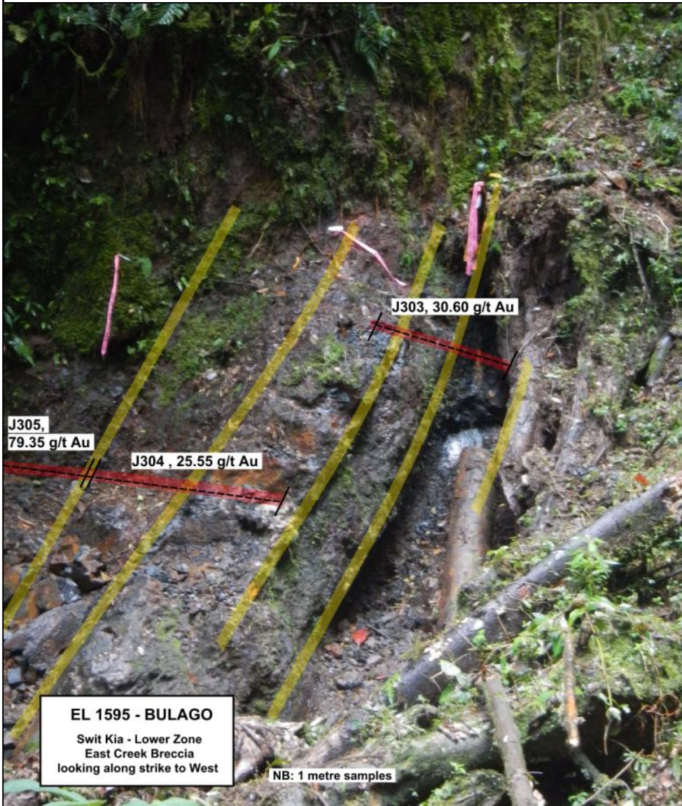
Photo 1. The East Creek breccia looking along strike to the WNW showing the moderate-high angle plunge or dip (?) to the SW, with 1.0m grading 79.35 g/t gold, within 3m grading 45.17 g/t gold (J303, J304 and J305). Unfortunately, the photo didn't capture the highest grade zone very well.
