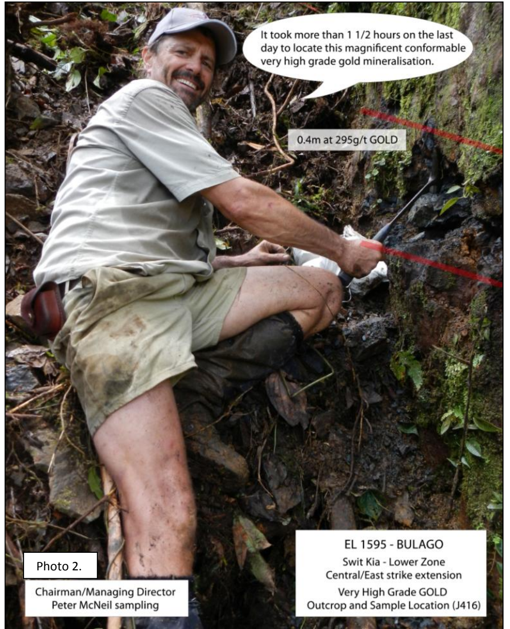
Photo 3. The highly sulphidic breccia and quartz veining with 0.40m grading 297 g/t gold outcrop (J 416).
