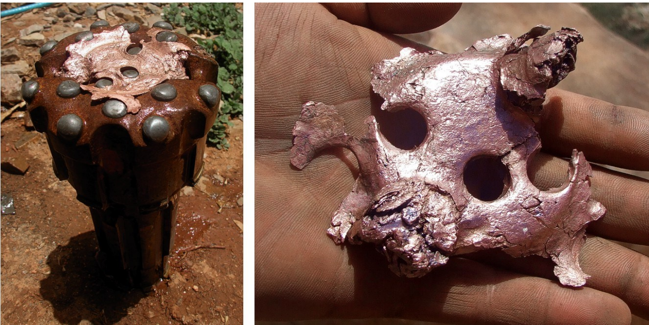
Figure 5: Example of large native copper nugget, possibly encountered in soft clay or friable oxide material and unable to return up the small (20mm) sample return holes at the end of the RC bit. Left; the remaining middle section appears to have been "stamped" out of a larger solid copper nugget that has been flattened, then cut through by the bit and right; underside of the copper "stamp" showing how the metal was pushed into the two sample return holes (top right & bottom left) and was unable to return to surface.
