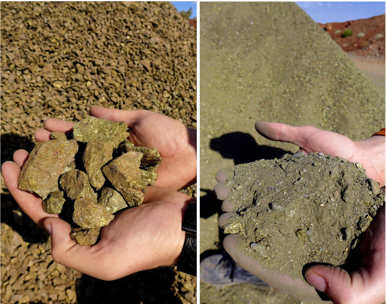
Figure 21: High-grade primary ore after passing through the mobile crushing circuit -80mm crush (left) and a chalcocite/chalcopyrite rich product after passing through the -20mm crush (right).
