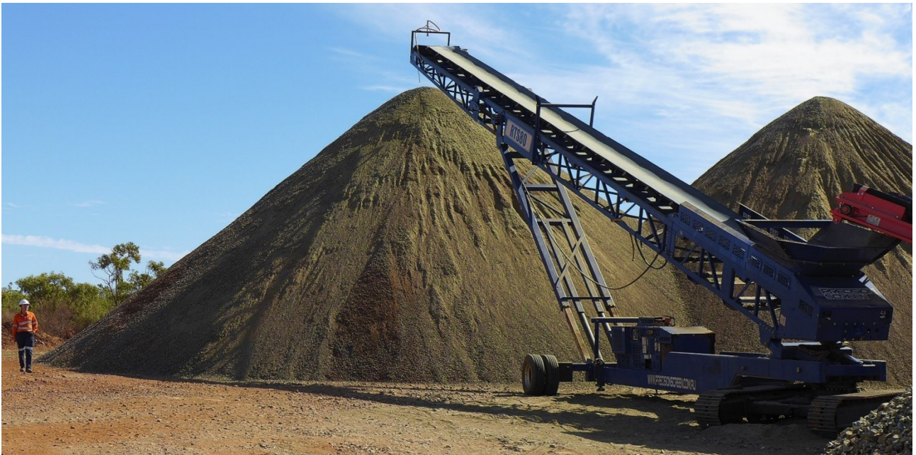
Figure 22: Primary ore DSO stockpile rich in chalcopyrite and chalcocite (above) and the Company's fully owned mobile crushing circuit (below) that performed above expectations during trial crushing of high-grade primary ore that was used for product testing and analysis. The crushing circuit is used predominately for generating crushed rock used for various end uses including road-base and stemming (used to pack blast holes).
