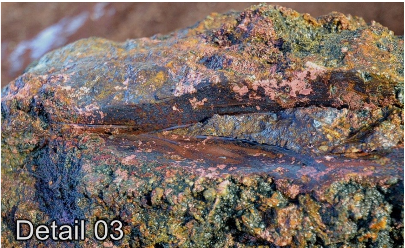
Figure 11: In sequence diamond saw cutting of sample wedge from large boulder estimated at ~2.5 tonnes, that was visually “unexciting” but found to contain significant copper including native copper (99.65% copper), cuprite (88.8% Cu) and chalcocite (79.9% copper).
