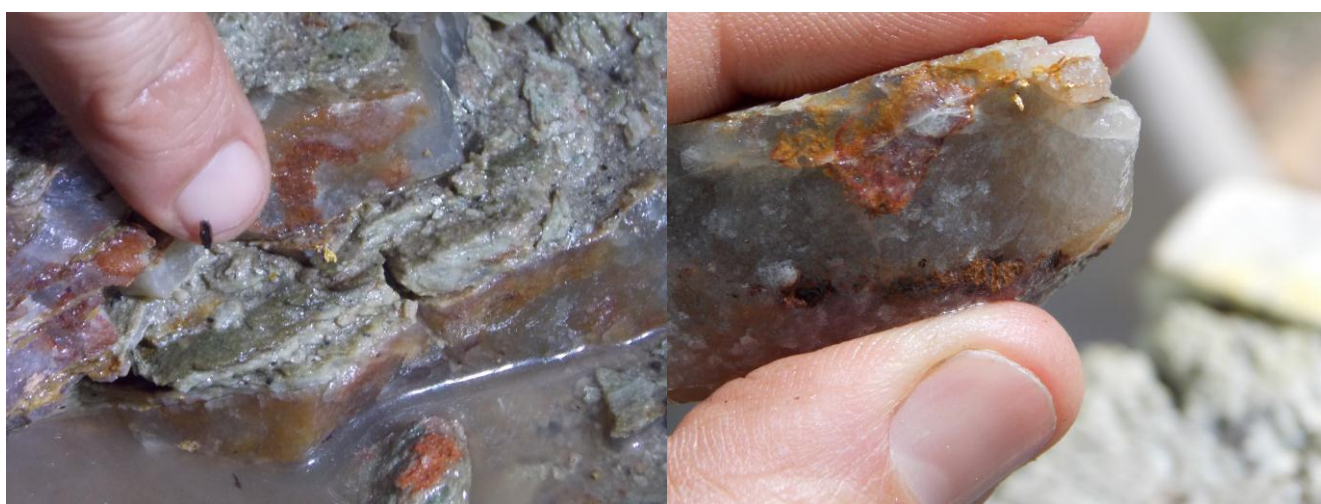
Figure 3. Cascavel provides the unique opportunity to see substantial amounts of visible gold in the walls of the exploration decline and hand samples. Left photo shows a nugget close to the decline floor and on the left side gold nuggets in the quartz vein.
