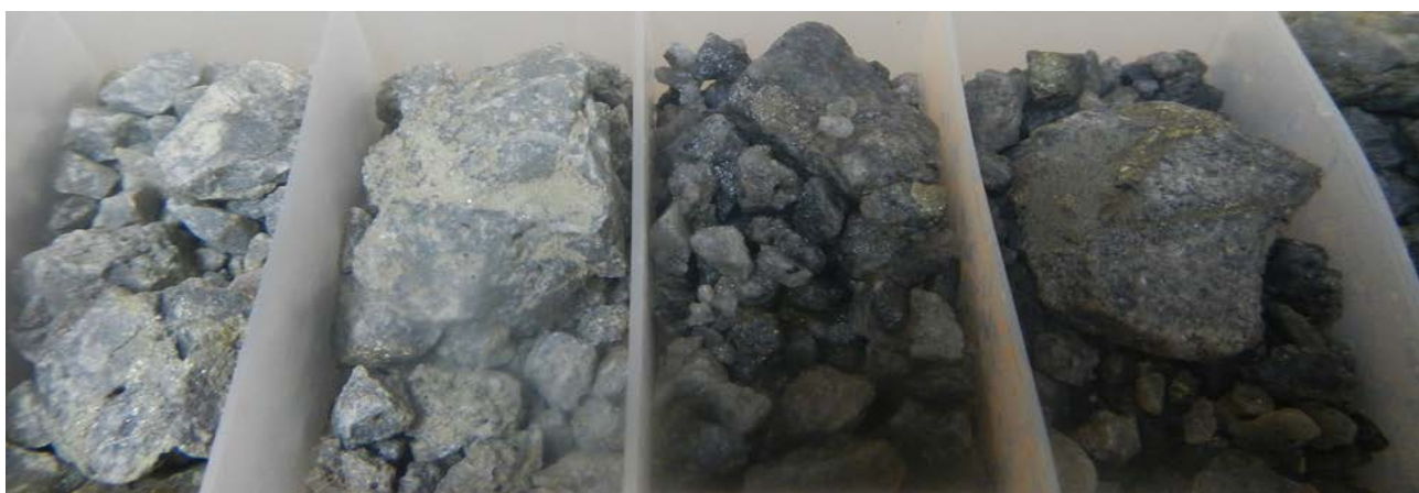
Plate 2. BGRC014 RC Chip Samples: 84m - 88m. Matrix sulphides in siliceous breccia (quartzite?)
