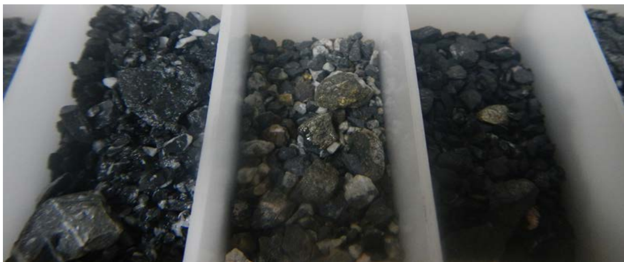
Plate 1. Hole BGRC004 RC Chip Samples: 113m - 116m. Laminated sulphides in carbonates & black shales
