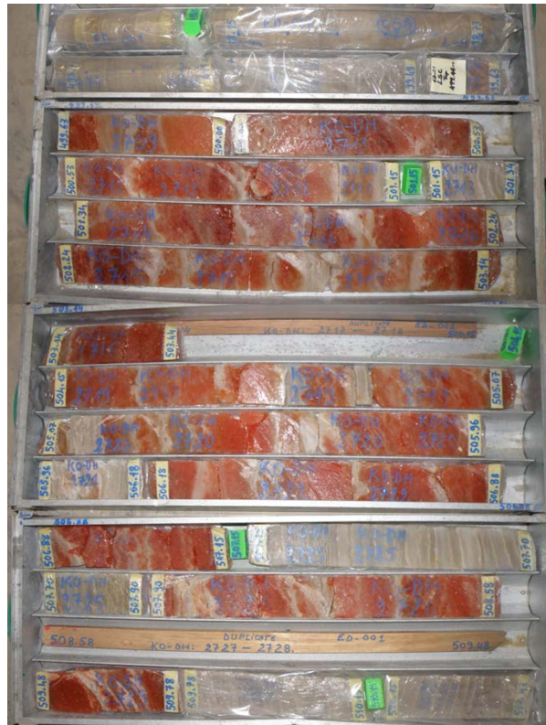
Figure 5. Lower Seam potash mineralization in ED_01. Carnallite from a depth of 499.48 to 509.78 metres (thickness of 10.30 metres) grading 18.63% KCl. Carnallite is orange in colour. Halite is white. The massive halite above and below the seam can be seen.
