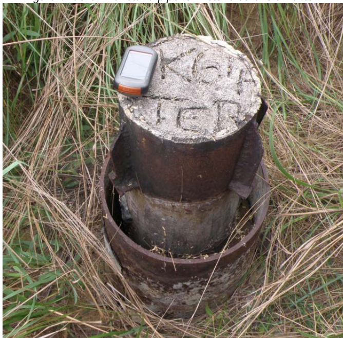
Figure 4. Collar with stand-pipe for historic borehole K64ter.
