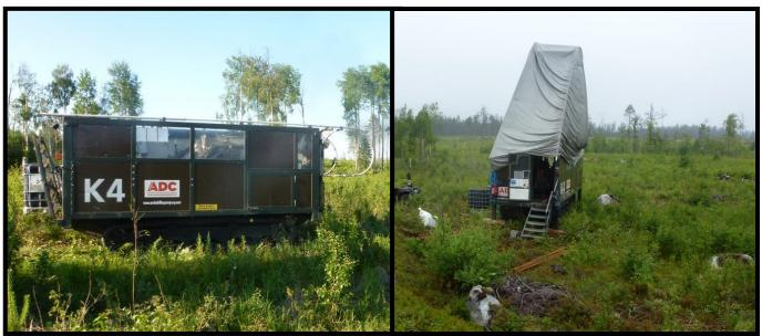
Figures 1 and 2. Small track diamond drill rig being utilised by Boss Resources for the current drill program with minimal footprint and impact on the surrounding environment.
