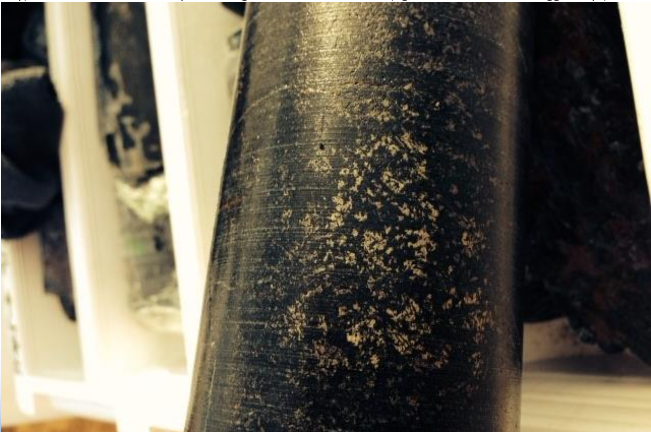
Figure 1. Disseminated sulphides in second reconnaissance drillhole SPBD0047.
