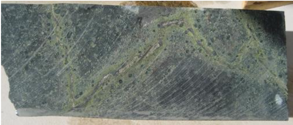
Quartz-pyrite vein with epidote selvage from upper section of GCHD469
