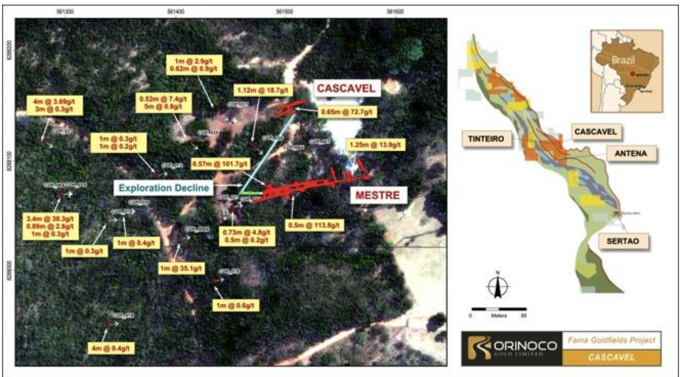
Figure 7. Location of Cascavel exploration decline. The proposed exploration decline (represented here in light blue) is a total of 90m in length. The results reported in this announcement represent the first 20m of that decline.
