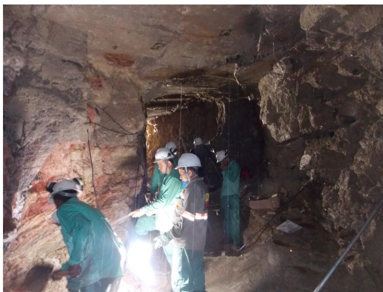
Figure 3. Cleaning the face of the exploration decline ahead of sampling.
