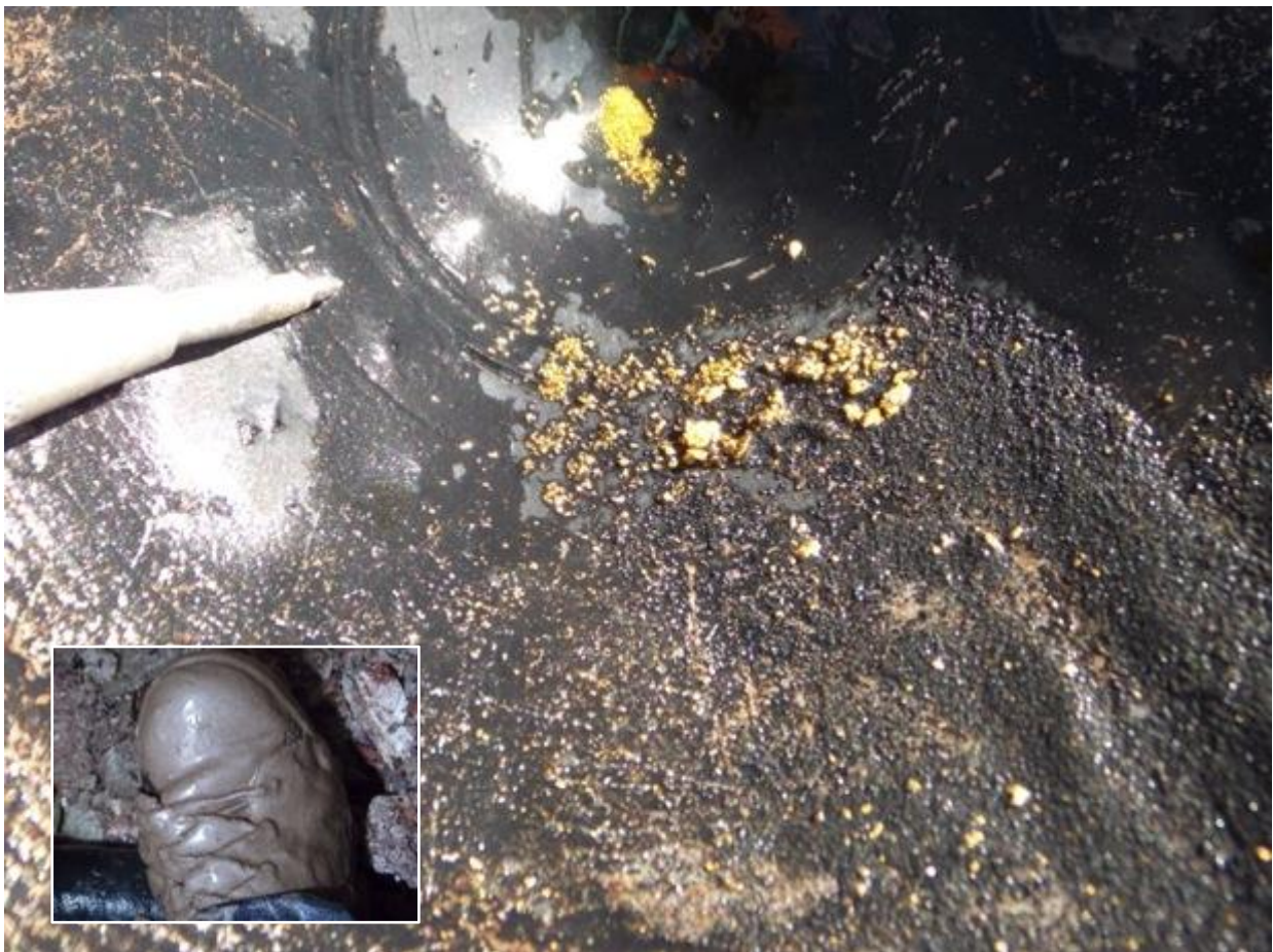
Figure 4. The strong (predominantly sericite) alteration around the high-grade shoots is strongly mineralised and results in a fine-grained mud that forms on the exploration decline floor (Inset). The panning of this mud reveals the strong mineralisation hosted in the alteration around the quartz veins/veinlets.
