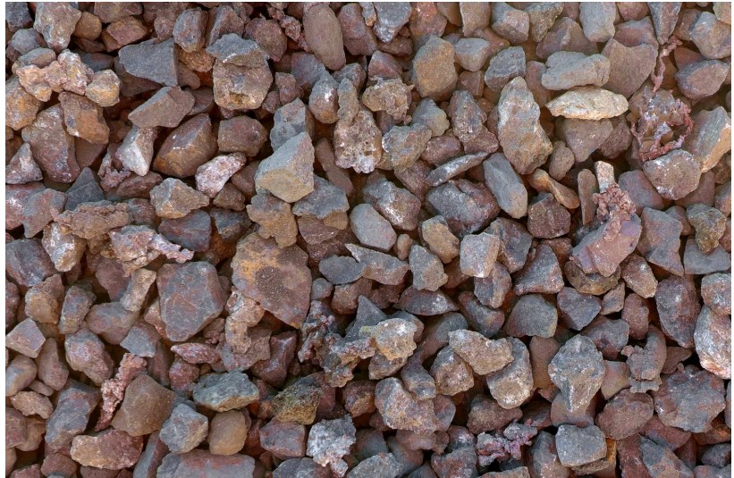
Figure 5: Close up of above crushed (-40mm) native copper ore stockpiles - ready for upgrading to a premium grade concentrate through the Company's new ore sorter, currently in its final stages of construction in Hamburg Germany. The above image shows coarse native copper nuggets, coarse and fine native copper in rock matrix, chalcocite, cuprite and various secondary copper species, visually estimated at 26% Cu in the above image.
