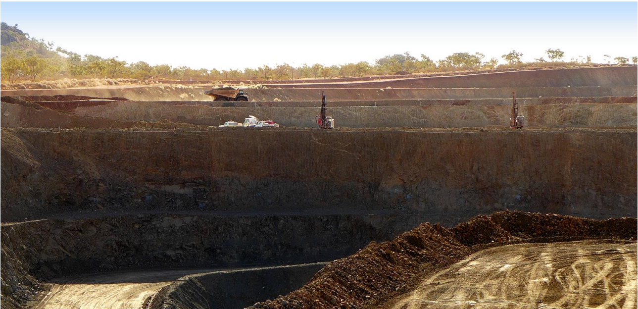
Figure 1: View to north-west showing all three stages of the Las Minerale Pit; Deepest pit is LM1; blast-hole drilling on the shoulder of the LM2 Pit floor and in the background; LM3 Pit (final pit) walls.
