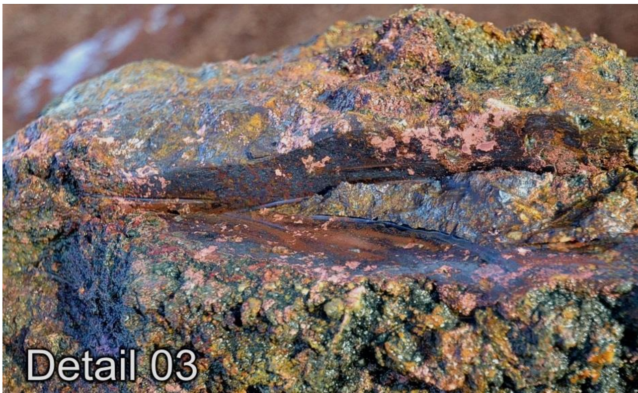
Figure 43: In sequence diamond saw cutting of sample wedge from large boulder mined at the start the LM1 Pit, estimated at ~2.5 tonnes, that was visually “unexciting” but found to contain significant copper including native copper (99.65% copper), cuprite (88.8% Cu) and chalcocite (79.9% copper).
