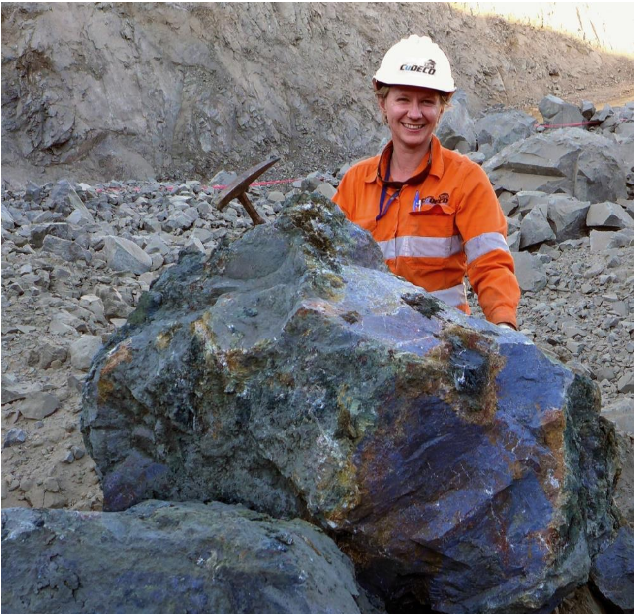
Figure 38: Large (~2.5 tonne) massive chalcocite boulder (chalcocite contains 79.9% Cu)...one of many excavated from the bottom of the LM pit. An impressive mix of supergene copper ore is being revealed during mining at Las Minerale, co-existing within a high-grade bonanza supergene environment associated with coarse native copper.
