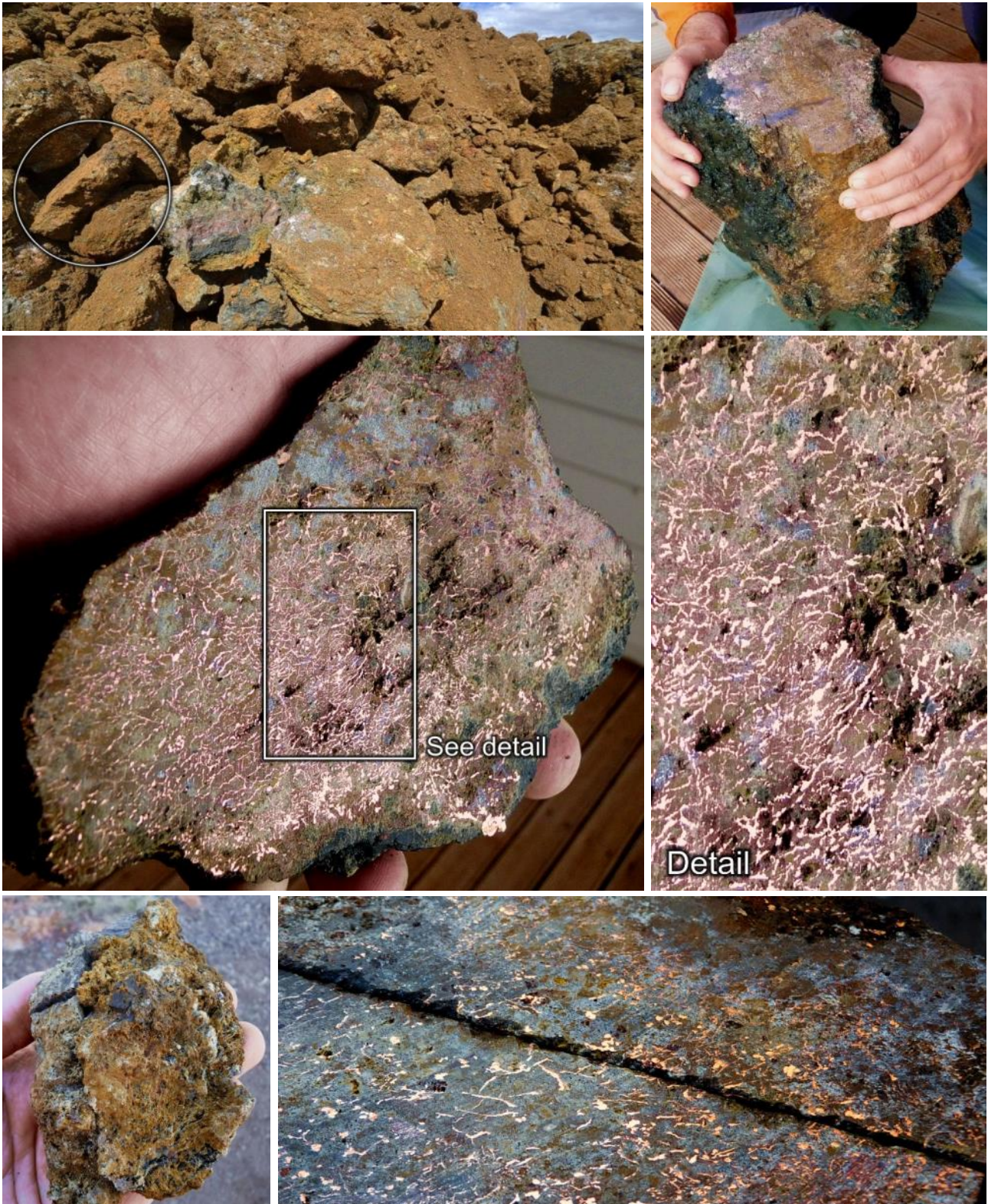
Figure 44: Small grab-sample of ore taken from native copper stockpile - rather unexciting on the outside, but once cut open the sample reveals the unique nature of the Las Minerale treasures, including native copper (99.65% Cu), cuprite (88.8% Cu) and chalcocite (79.9% Cu). The grab sample was selected by hand, so by necessity (due to the high density high-grade native copper ore), was limited to what could be easily carried. This grab sample from the stockpiles, whilst small, weighed well over 50kg.
