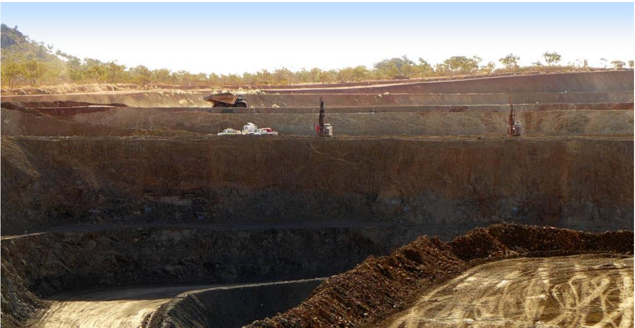
Figure 4: View to north-west showing all three stages of the Las Minerale Pit; Deepest pit is LM1; blast-hole drilling on the shoulder of the LM2 Pit floor and in the background; LM3 Pit (final pit) walls.
