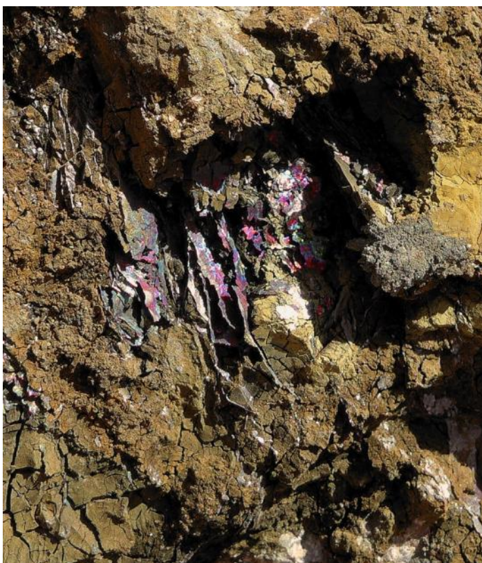
Figure 48: Selection of native copper specimens from the native copper stockpile; Sheet native copper (above), native copper sheets in rock-matrix (bottom right) and nuggetty agglomerates with chalcocite (grey-blue) and tenorite (blue-black), left.
