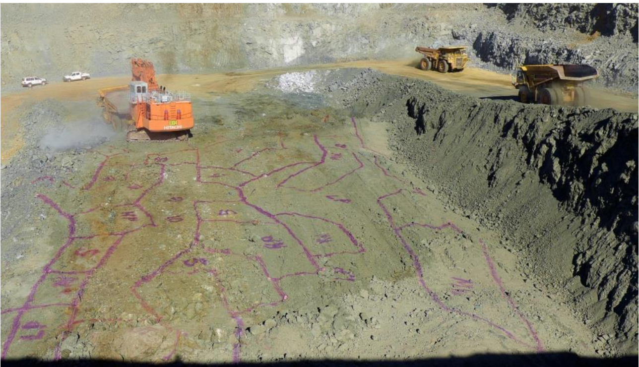
Figure 40: LM1 Pit at the RL170m level (~45m from surface), showing the LM1 pit-floor mark-up at RL170. The mark-up shows the first hints of high-grade ore (+10% copper) emerging through the very top of the DSO ore zone. The average grade of the +10% zone in this area is 14.6% Cu (with highs in the range 22% Cu), and the average grade of the +5% zone is 8.2% Cu (highs of 9.8% Cu), based on blast-hole sampling. Blast-hole sampling correlates well with the resource model. Recent bulk-sample test recovery of native copper ore (estimated from blast-hole sampling at 0.5% Cu - that also correlated well with the resource model) resulted in a 400% increase in grade after processing generated significantly more copper than estimated, using the Company's trial ore-sorter. The trial results provide evidence not all native copper is being recovered during drill sampling (especially coarse native copper in clays and soft or weathered rock matrix), resulting in grade estimates less than are actually being mined.
