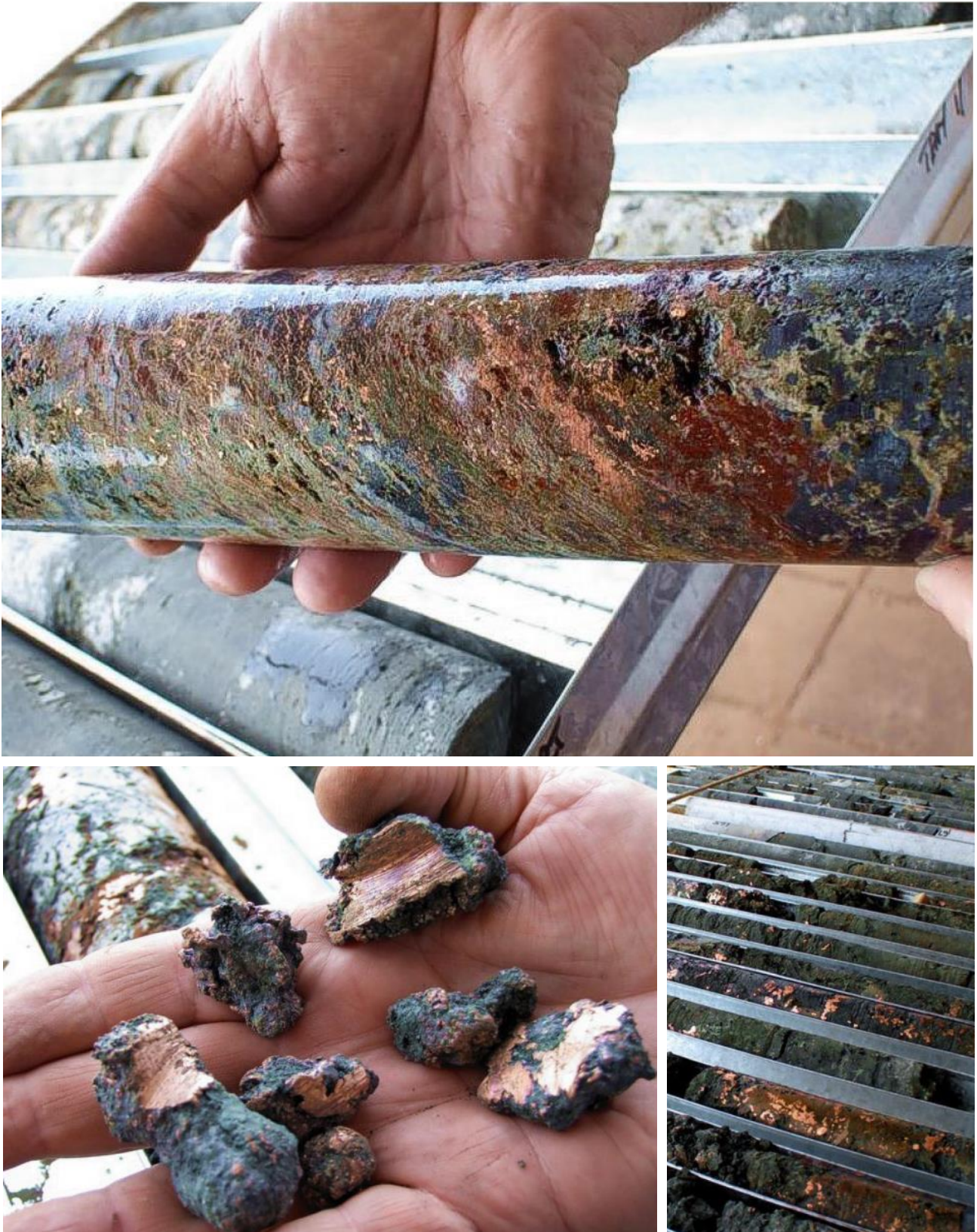
Figure 36: Examples of coarse native copper and chalcocite in metallurgical drill core from the Las Minerale Bonanza zone
