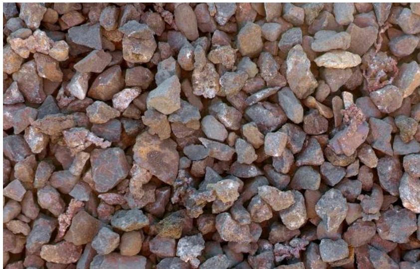
Figure 8: Close up of above crushed (-40mm) native copper ore stockpiles - ready for upgrading to a premium grade concentrate through the Company's new ore sorter, currently in its final stages of construction in Hamburg Germany. The above image shows coarse native copper nuggets, coarse and fine native copper in rock matrix, chalcocite, cuprite and various secondary copper species, visually estimated at 26% Cu in the above image.
