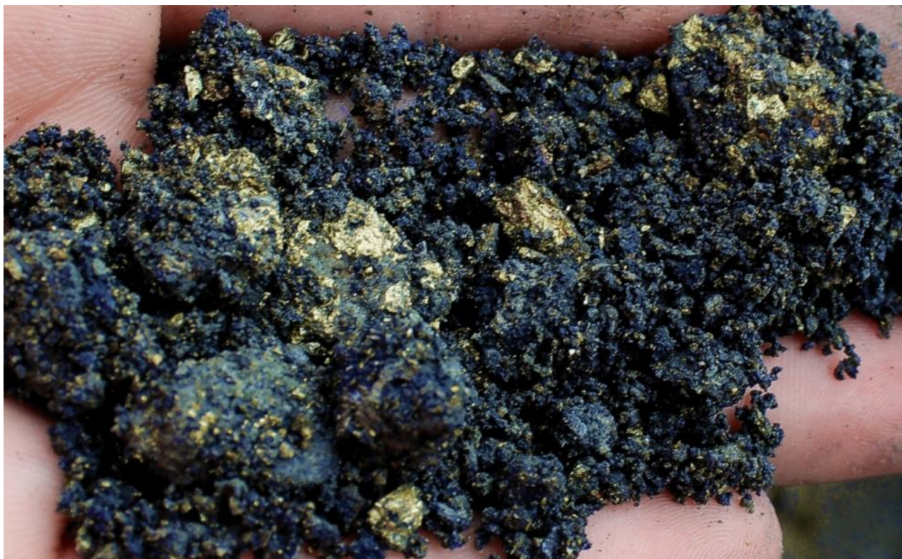
Figure 45: Example of chalcocite rich clays co-mingled with chalcopyrite and resembling the consistency of soil, with copper grades ranging between 24-56% Cu from 30 random XRF spot-checks in the pit.
