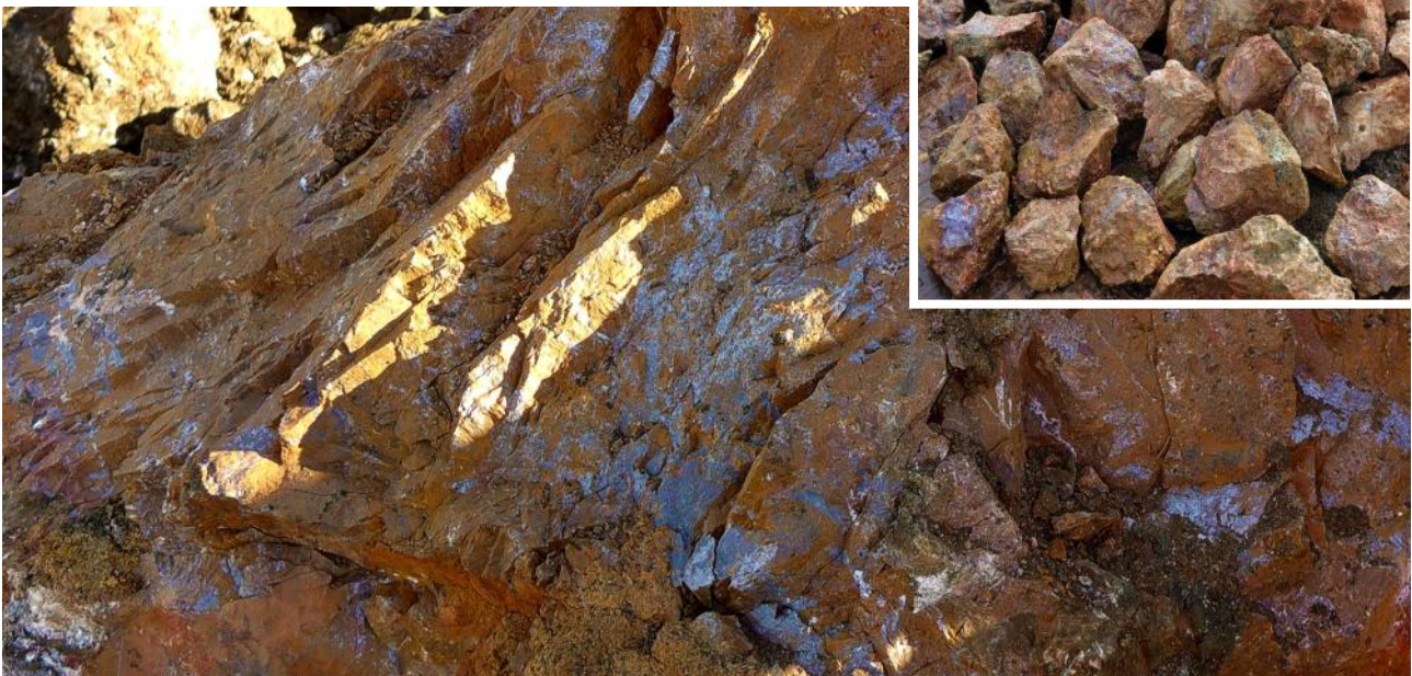
Figure 64; high-grade copper ore from the LM1 Pit - iron-rich yellow jaspilite rock matrix impregnated with massive and vein infill chalcocite (79.9% Cu), massive cuprite (88.8% Cu) and fine to coarse native copper species (99.65% Cu) - inset shows similar jaspilite after crushing through the mobile crusher, accessed in the original box-cut pit.
