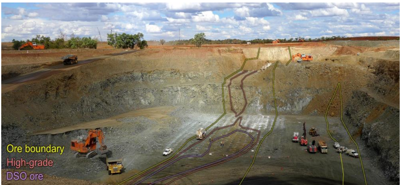
Figure 54: LM1 Pit at RI180, with indicative ore outlines shown - high-grade native copper ore suitable for DSO is highlighted.
