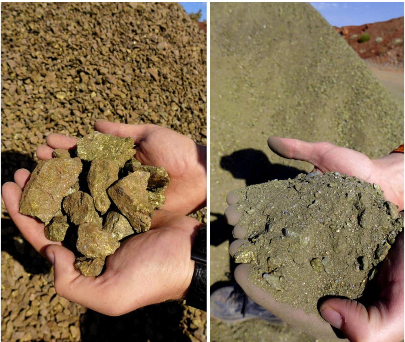
Figure 53: High-grade primary ore after passing through the mobile crushing circuit -80mm crush (left) and a chalcocite/chalcopyrite rich product after passing through the -20mm crush (right).
