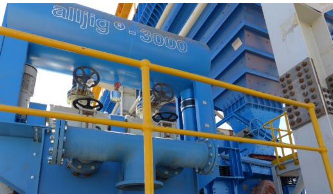
Figure 11: Gravity Jig Building - from top to bottom; native copper metal screens, feed bins and light screens and continuous alljig® units (left and right)
