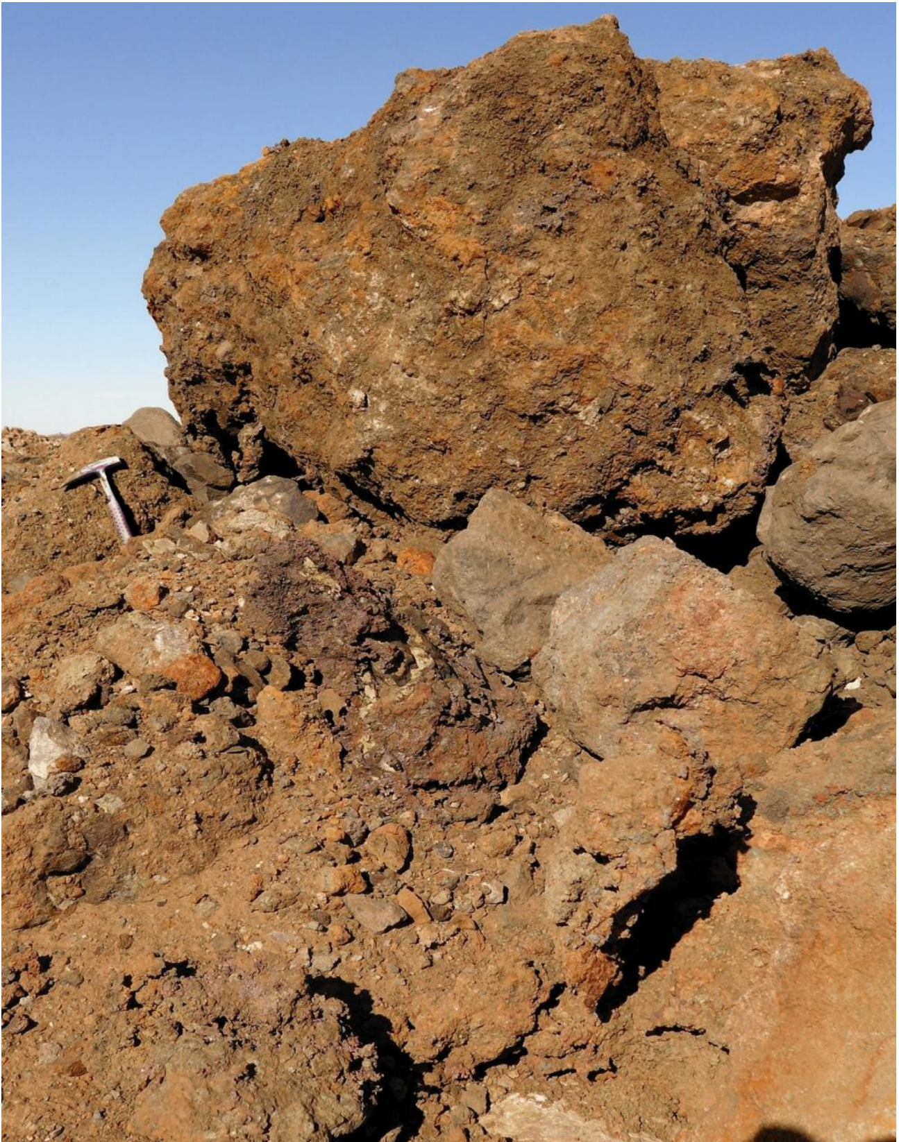
Figure 42: Large coarse native copper masses recently loaded onto the DSO stockpiles - this one estimated at over 4 tonnes.
