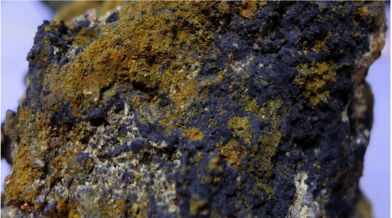
Figure 50: Tenorite (79.6% Cu - blue/black) mantling cuprite (88.8% Cu - not visible) and beneath that native copper (99.65% Cu - not visible).
