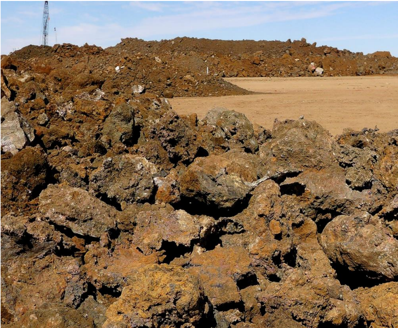
Figure 28: Large, (up to 4 tonne) coarse native copper masses building on the various ROM DSO stockpiles (native copper contains 99.65% copper metal). Crushing circuit being modified to screen and process larger than expected masses of native copper for DSO.
