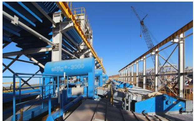
Figure 11: Gravity Jig Building - from top to bottom; native copper metal screens, feed bins and light screens and continuous alljig® units (left and right)
