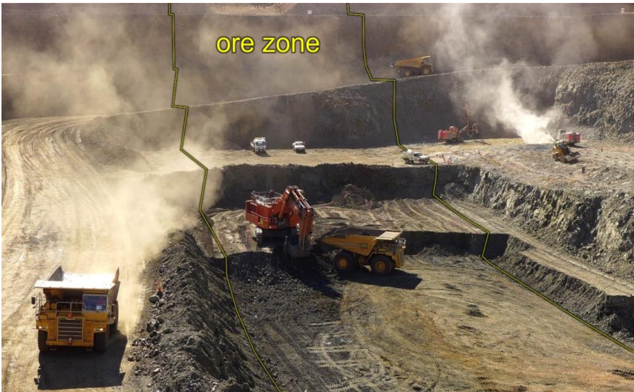
Figure 1: Stage-1 Las Minerale Pit (LM1 Pit) reaches the RL175 level - accessing very high-grade coarse native copper & chalcocite.
