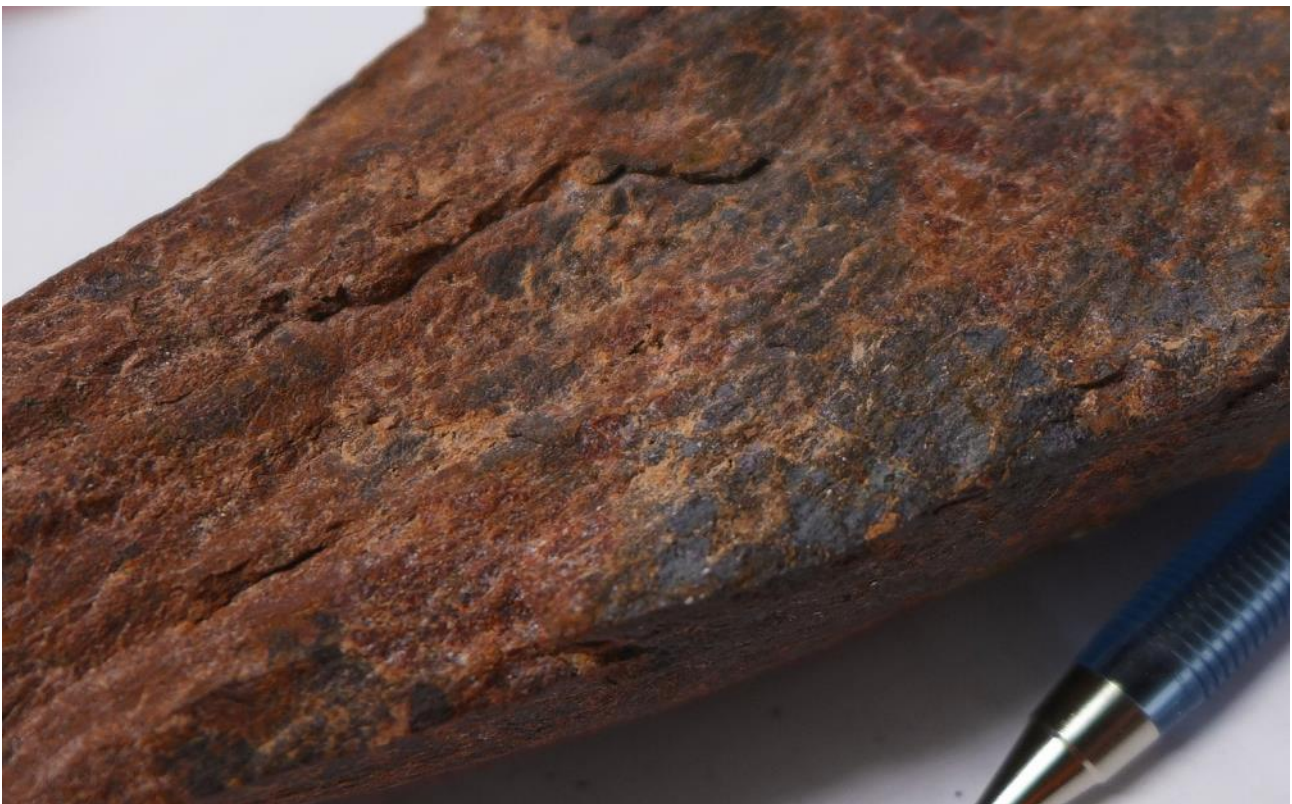
Figure 49: Top image; Minor native copper (99.65% Cu - not visible) surrounded by cuprite (88.8% Cu - metallic red/grey), azurite (55.3% Cu - blue), and malachite (57.5% Cu - green)...as the high-grade native copper reduces into various copper species due to the influence of weathering. Bottom image; a version of cuprite known as tile ore (88.8% Cu), named after its colour and the sound it makes when broken (similar to roof tiles breaking).
