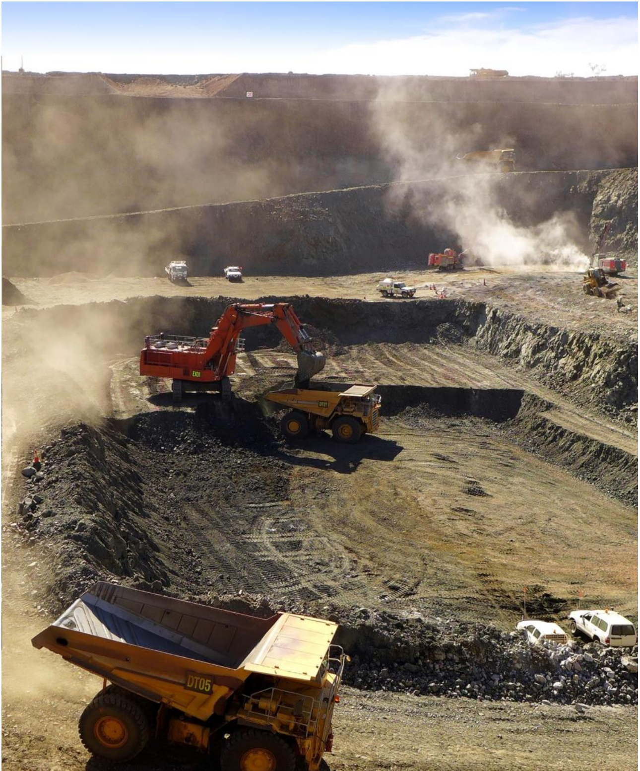
Figure 58: Mining of the very high-grade native copper ore in the LM1 Pit (foreground) as the next blast is loaded (right background). Whilst the truck under the digger is being loaded, another truck arrives (foreground ramp) and the previously loaded truck exits via the background ramp fully loaded. At surface, the truck loaded prior to that is heading to the stockpiles. This cycle continues all day, with 4 trucks per digger ensuring maximum cycle efficiencies.
