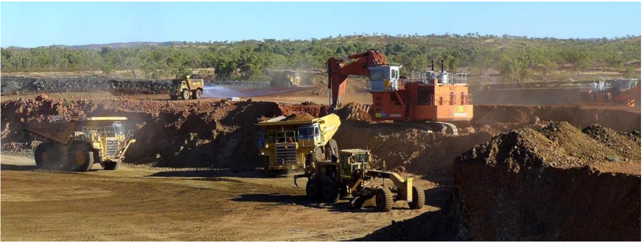
Figure 59: Mining concurrently underway at the north-west of the LM3 Pit (Final pit), accessing ore and waste previously blasted and remaining in-situ.
