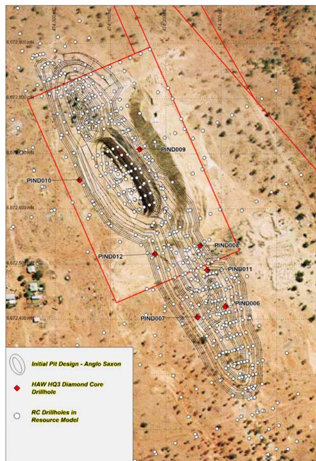
Figure 2. Initial Pit Design and location of Diamond Drill Holes – Anglo Saxon Deposit
