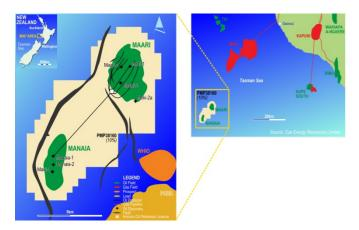
The Maari Growth Projects Program, incorporating 4 new production wells, 1 new injection well and a workover of the existing MR2 dual lateral production well, designed to enhance production rate and oil recovery from the Maari and Manaia fields, progressed in the quarter.
