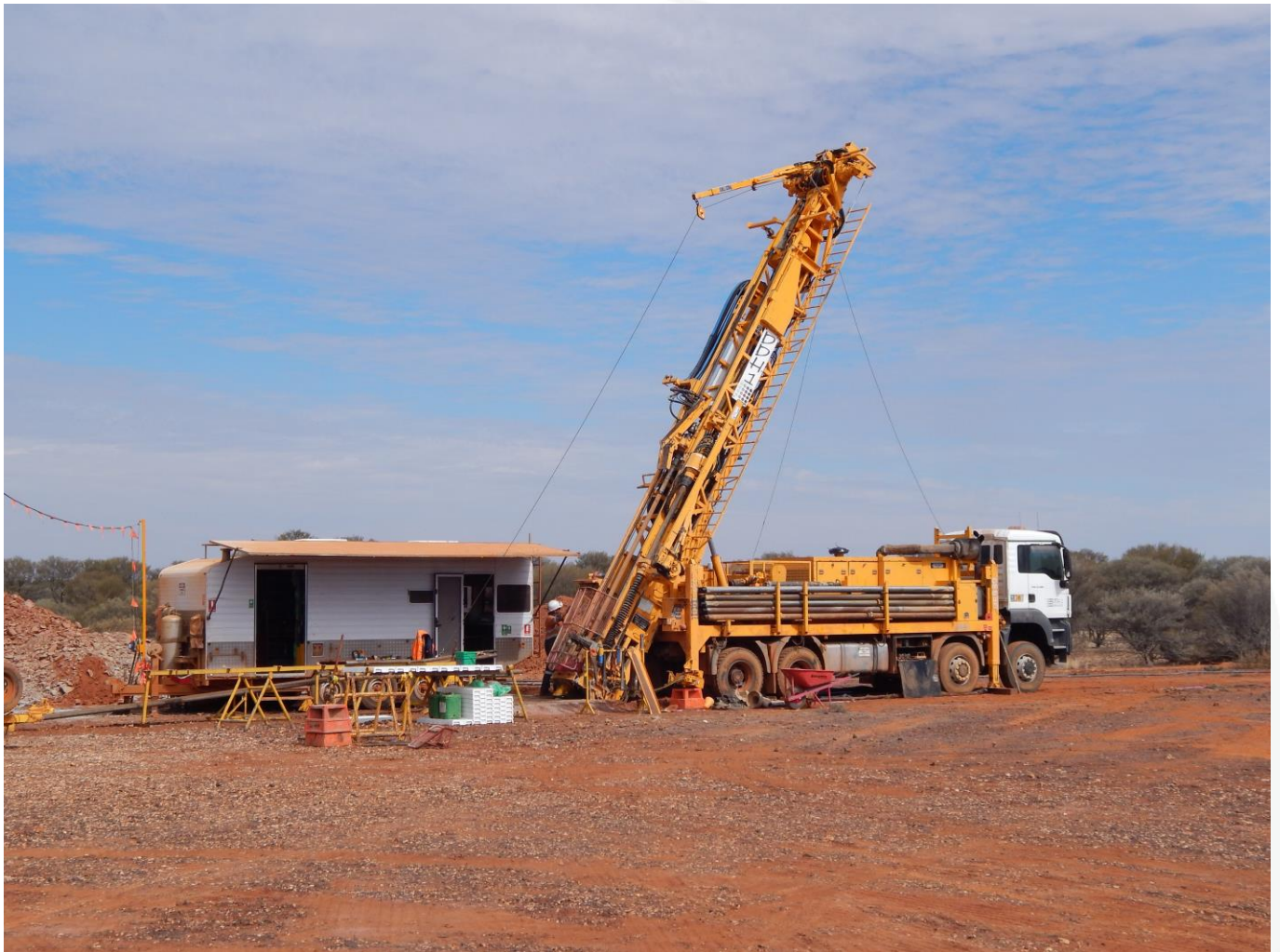
Figure 1: The diamond rig has commenced drilling the maiden hole (hole number SMDD001) at Australian Mines' Simmons prospect. This drill hole is designed to test the source of the bedrock conductor identified adjacent to an historic nickel-in-soil anomaly.
