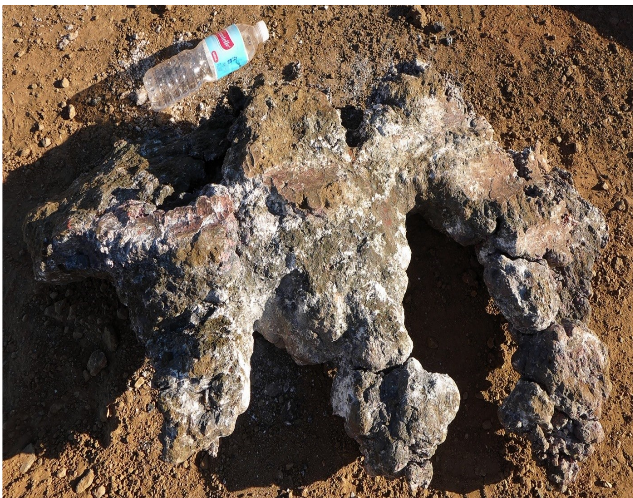
Figure 7: Large 130kg predominately native copper mass, with marks from the jaw crusher imprinted onto its surface. See following page for further details.
