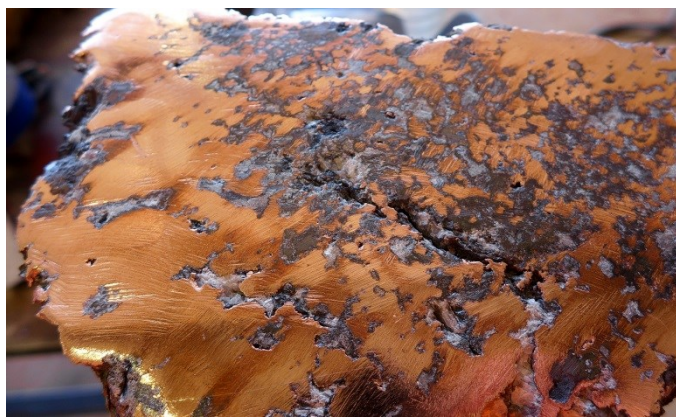
Figure 8 (above); large predominately native copper mass weighing ~130kg, with marks from the mobile jaw crusher imprinted onto its surface. This sample did not appear particularly solid at first glance (see Figure 7 previous page), but once a thin layer of surface rock was removed with a hammer, near solid copper metal was revealed.
