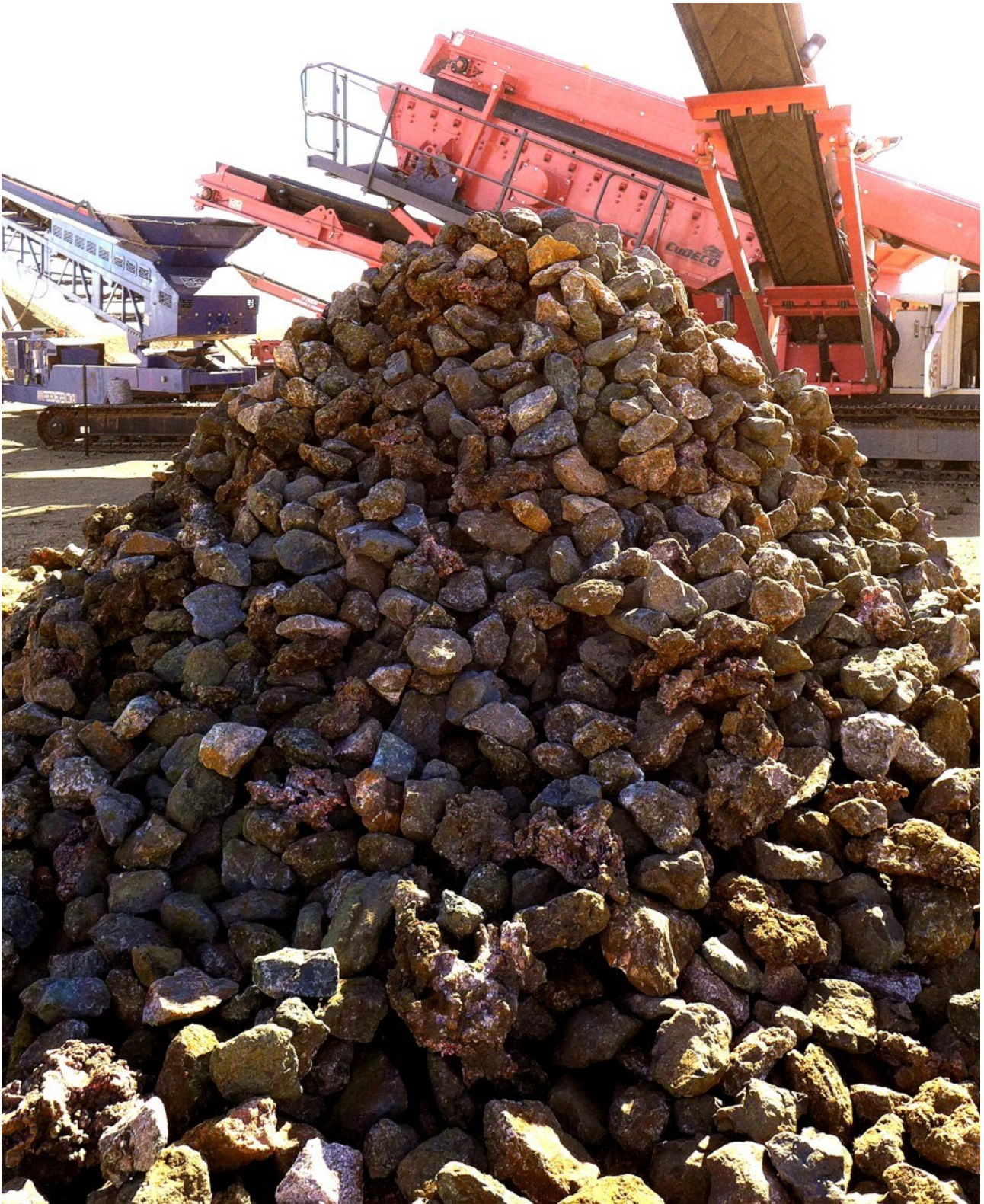
Figure 5: Scalped coarse DSO (+110mm) product includes coarse native copper nuggets, coarse and fine native copper in rock matrix (native copper contains 99.65% Cu), chalcocite masses, blebs and infill (79.9% Cu), cuprite (88.8% Cu) and various secondary copper species, visually estimated at ~30% Cu in this batch.
