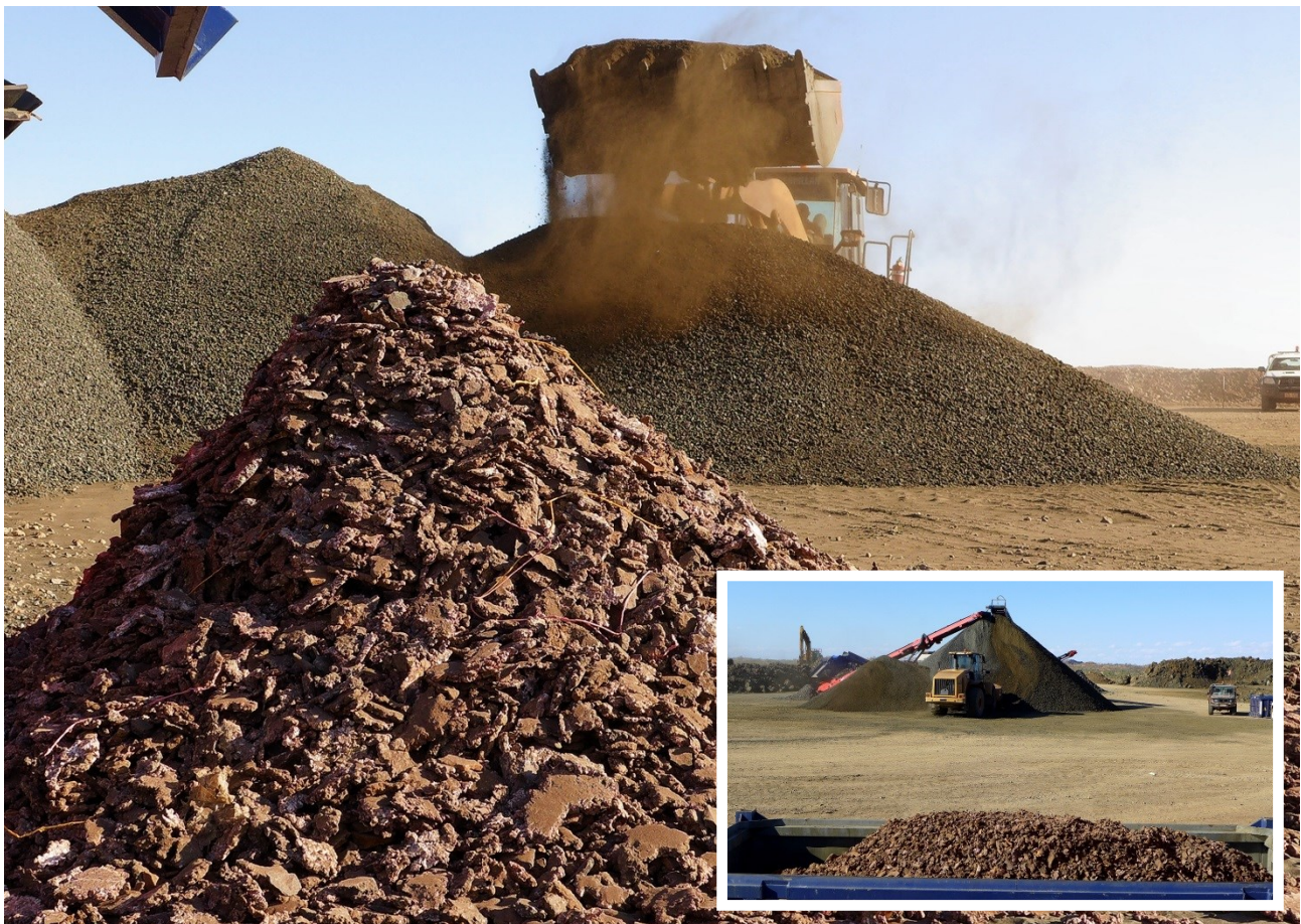
Figure 3: High-grade DSO (+40mm) scalped off the crusher screens. Predominately native copper (99.65% Cu), with minor cuprite (88.8% Cu) and chalcocite (79.9% Cu) and various supergene copper species. Inset; crushed product under the -40mm conveyors and +40mm scalped native copper DSO product in containers in foreground.
