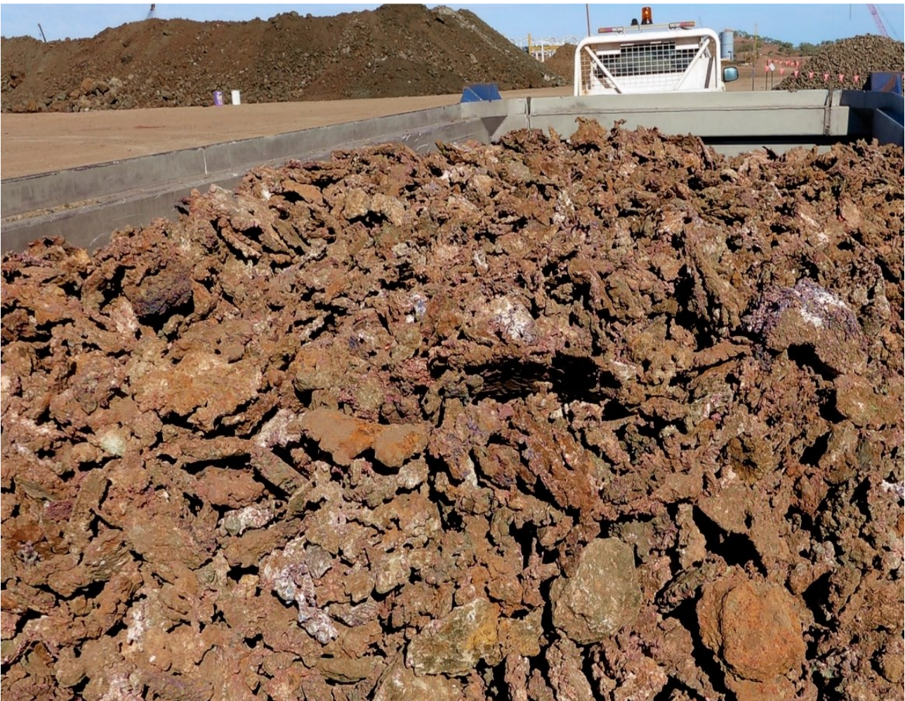
Figure 1: Container full of DSO straight from the crusher screens estimated 85-95% Cu, (+40mm—110mm)
