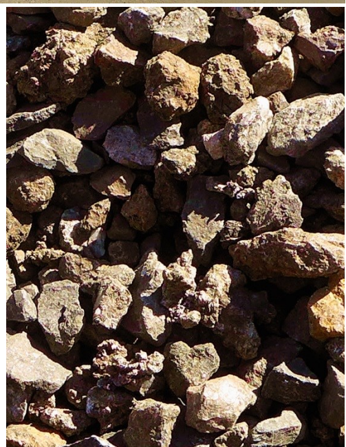
Figure 4: High-grade crushed ore (after removal of +40mm NCu) estimated (10-15% Cu - see detail above and right), stockpiled for processing through the Company's ore-sorter, loaded into containers for shipping. The crushed ore consists of native copper (99.65% Cu), with cuprite (88.8% Cu), chalcocite (79.9% Cu) and various supergene copper species.
