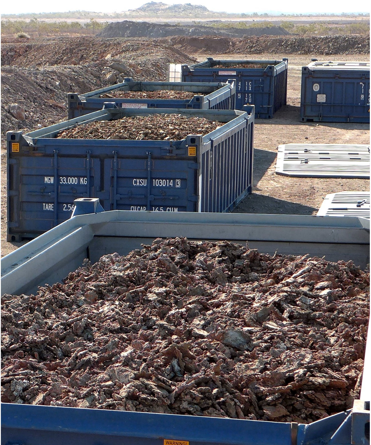
Figure 2: High-grade DSO (+40mm) visually estimated at 80-90% Cu, scalped off the crusher screens and loaded into containers ready for shipment. Each container holds between 22-25 tonnes of predominately native copper (99.65% Cu), with cuprite (88.8% Cu), chalcocite (79.9% Cu) and various supergene copper species.
