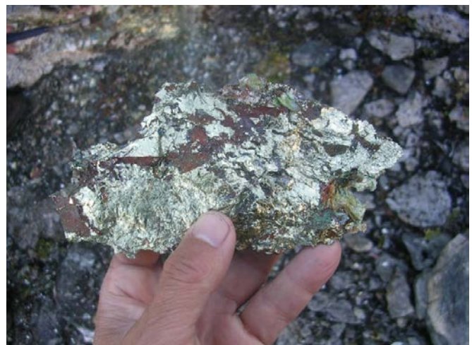
Figure 2. (a) Outcrop discovered by the NGU; (b) specimen mineralisation (chalcopyrite, steatite) at surface.
