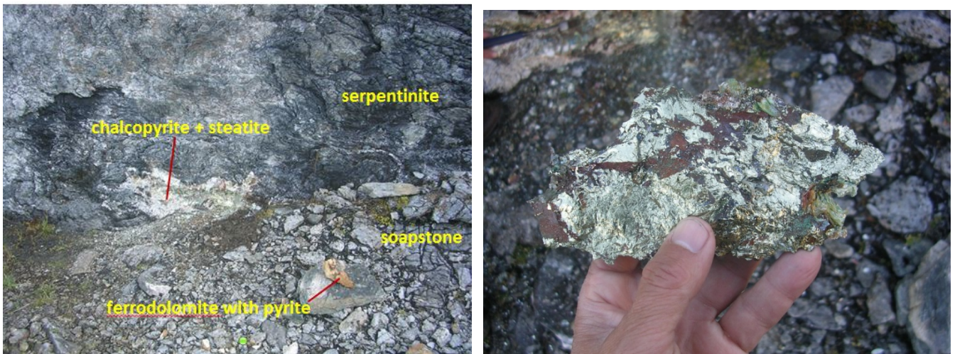
Figure 6. (a) Outcrop discovered by the NGU; (b) specimen mineralisation (chalcopyrite, steatite) at surface.
