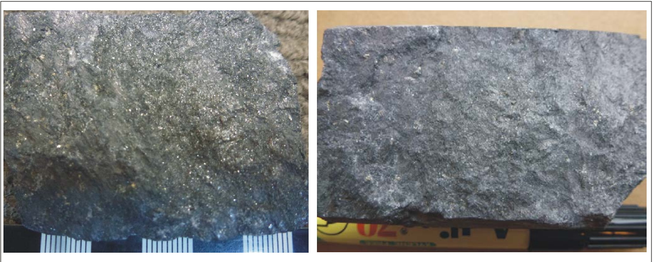
Figure 1. Drill core samples of the graphite mineralisation (graphite-bearing pelitic shales) intersected drillhole Boss-2 at the Skogtrask Project, Sweden.
