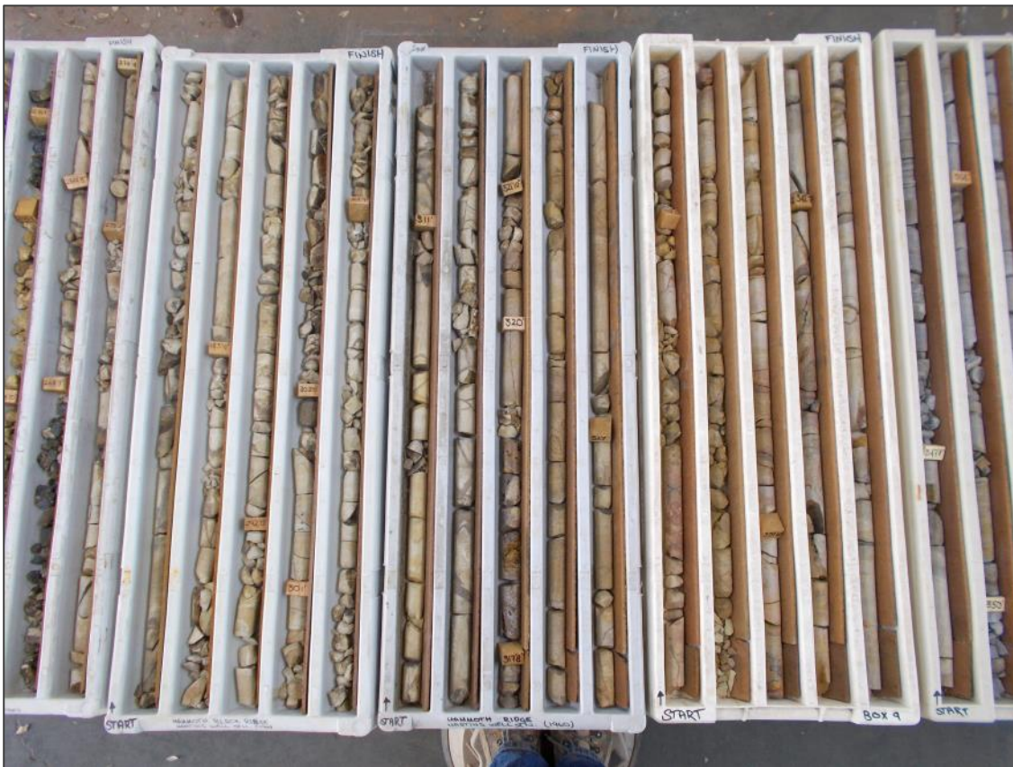
Gossan footwall siltstones in DD-2
