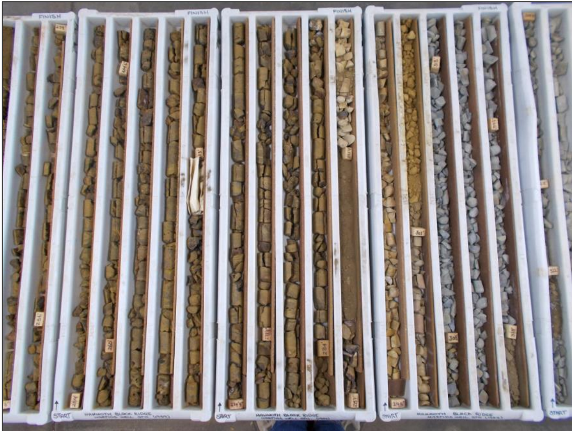
Iron Gossan and footwall siltstones in DD-1
