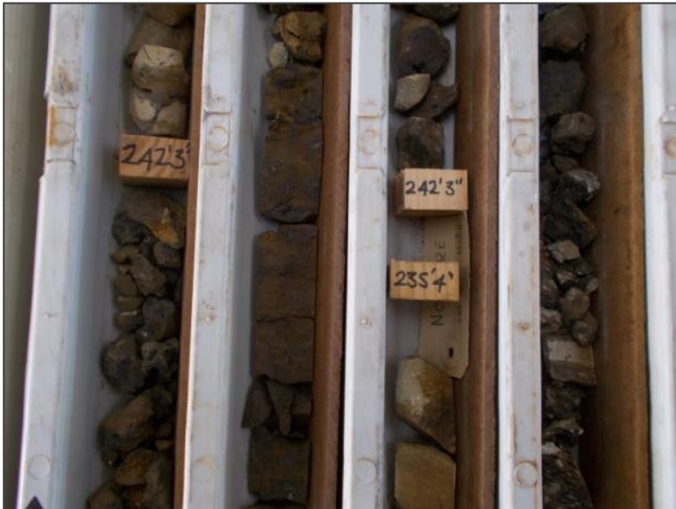
Figure 7 DD-2 - Gossan material
