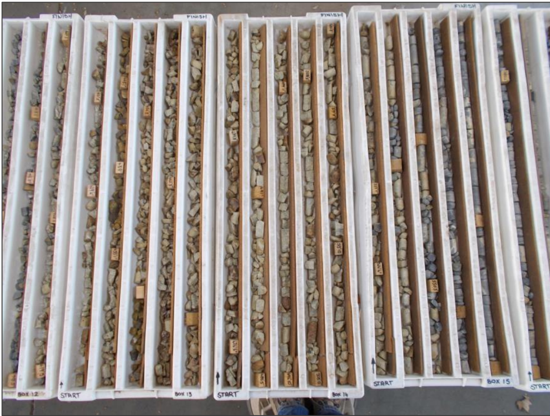
42 metres thick siderite unit with minor iron structures and disseminated chalcopyrite mineralisation DD-2
