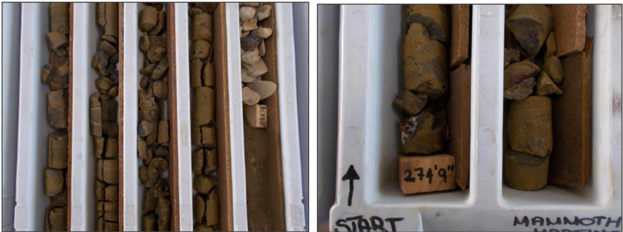
Figure 5 Gossan structure in DD-1 core More complete core photos are shown in the Appendix.
