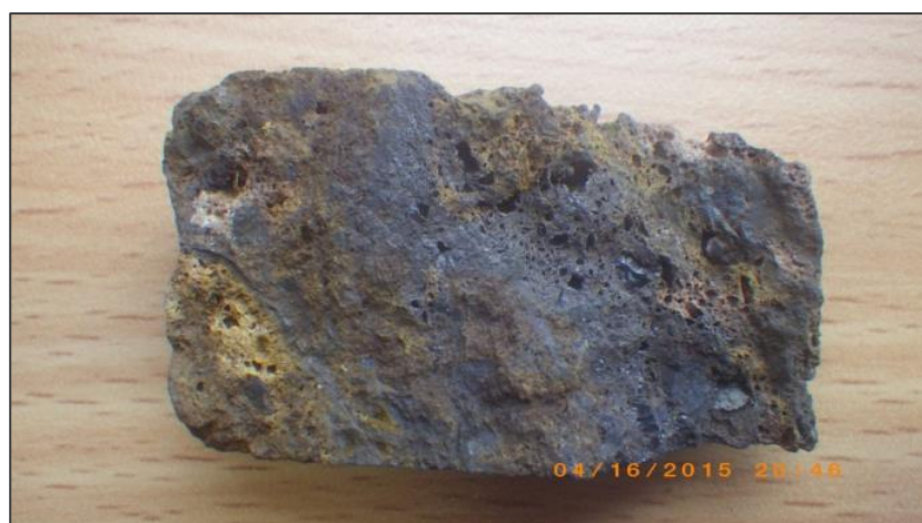
Figure 1 Diamond Hole DD-1 Iron Gossan sample with ex-sulphide boxwork textures
