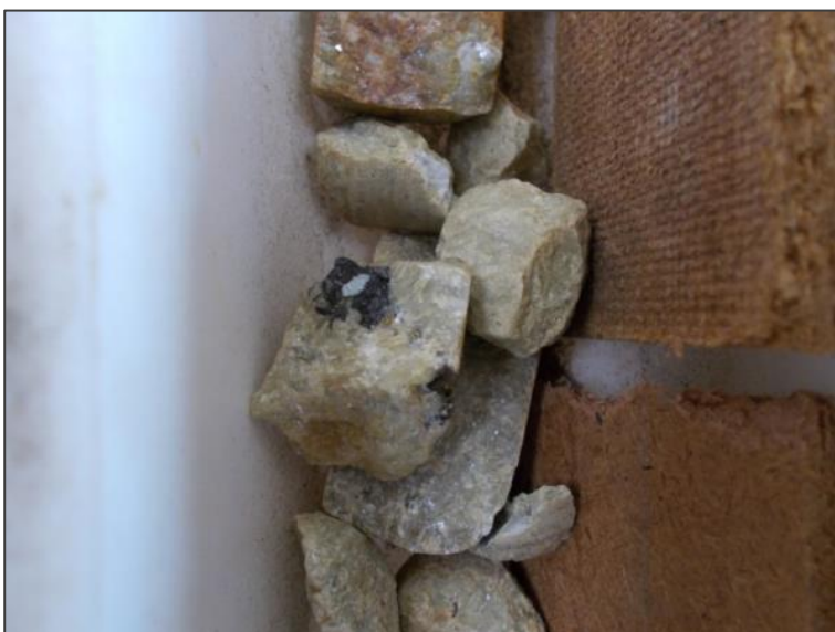
Figure 8 DD-2 Chalcopyrite aggregate in siderite
