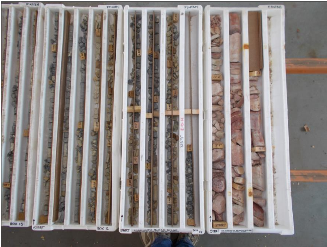
Lower siderite units at end of DD-2. Short hole DD-3 of unknown location on the right.
