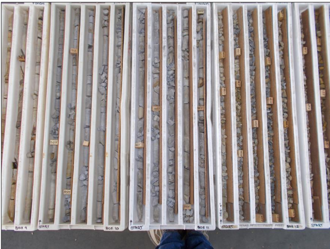
Commencement of siderite unit at 385'4" in DD-2
