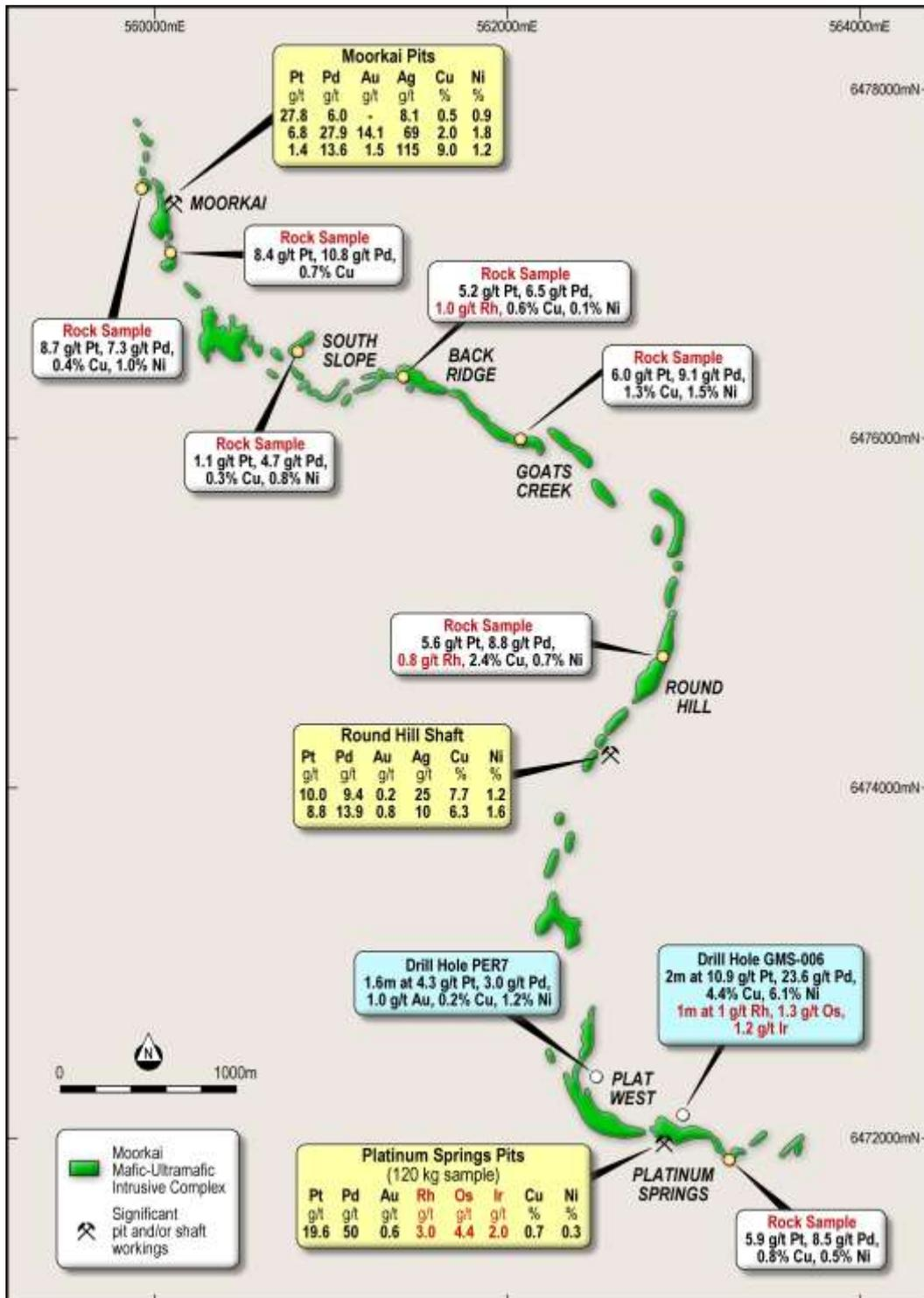
**Figure 1.** PGM-copper-nickel assays at the Moorkai Intrusive Complex
