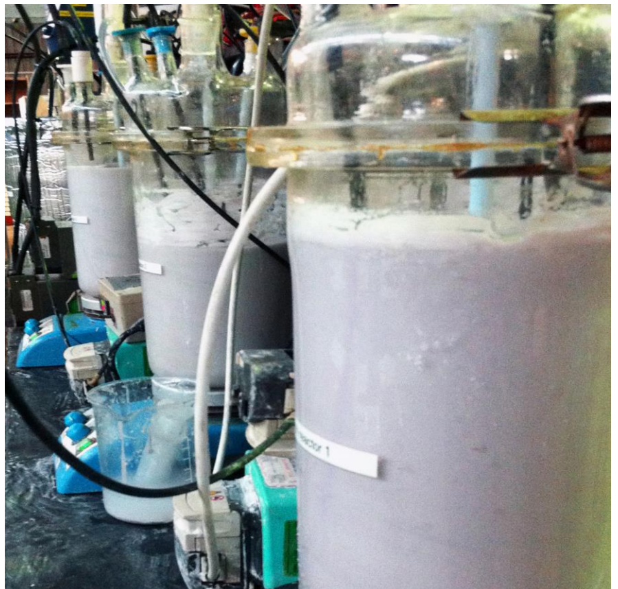
Processing Lepidolite Hill lithium micas in the Strategic Metallurgy mini-plant
