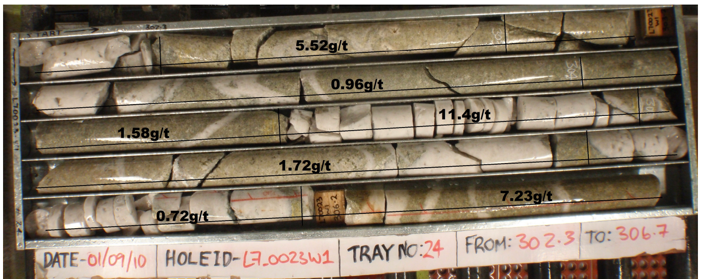
Figure 4-3: Ladder Style (Stockwork) Mineralization Example – Hole L7_0023W1
