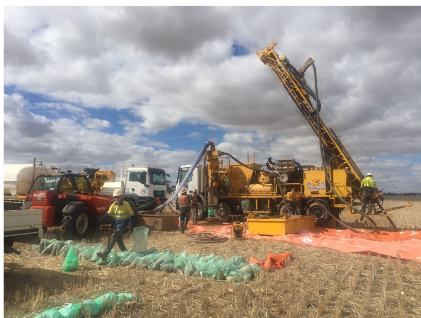
Reverse Circulation drilling operations at Alford West
