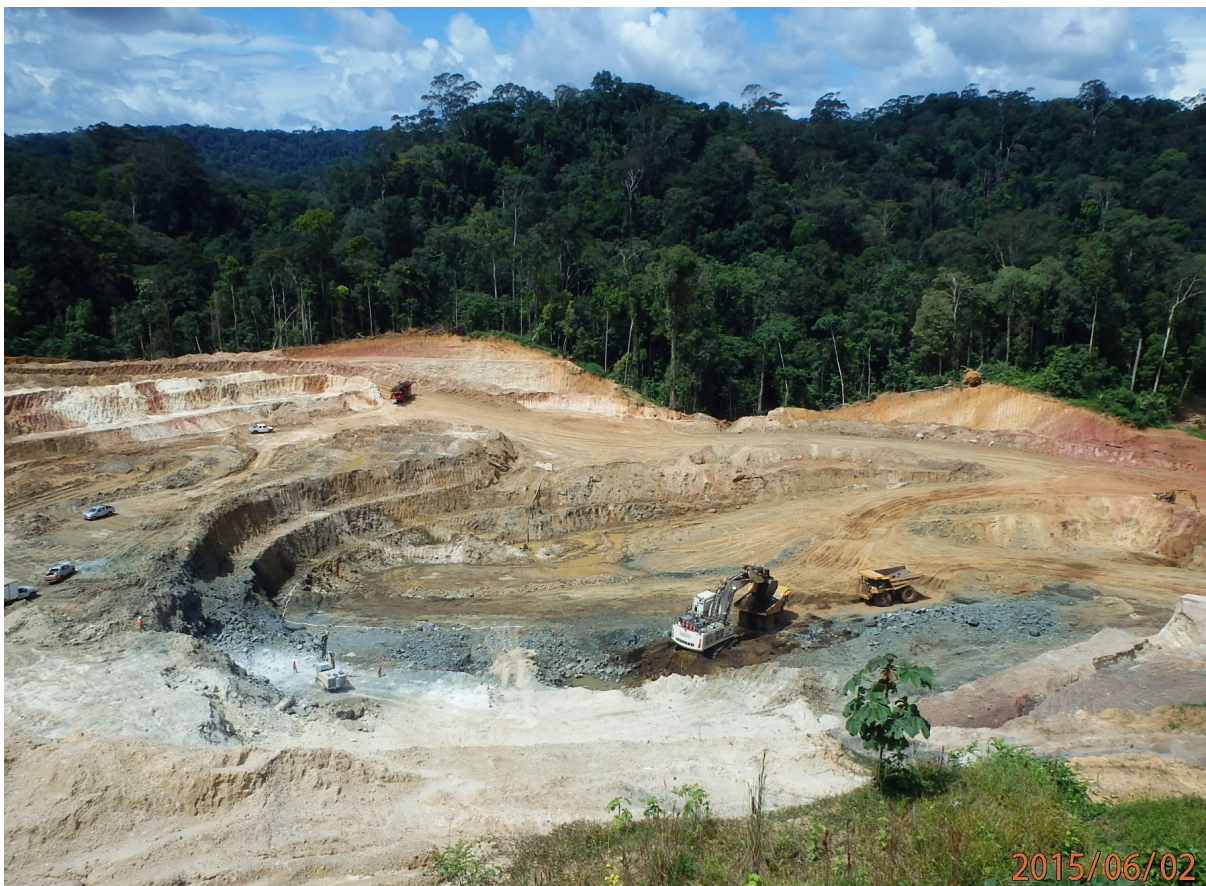
Photo 1. Mining high grade ore (2.2 g/t gold) at Urucum pit with a 250T excavator on June 2, 2015
