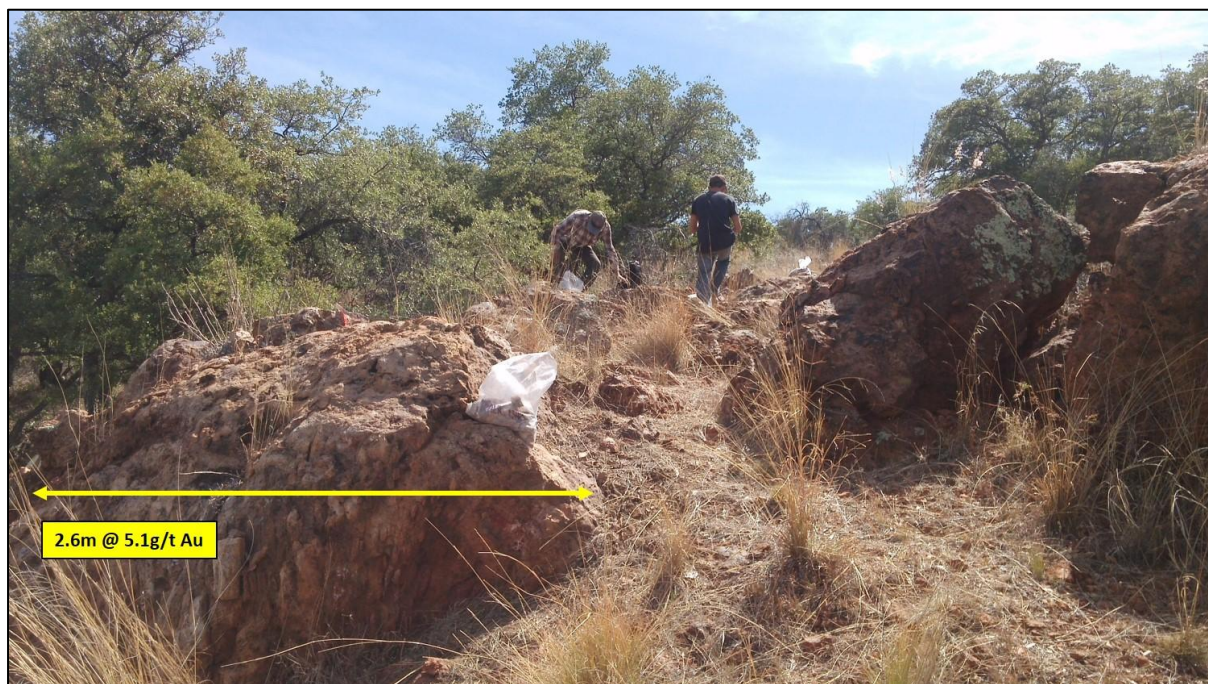
Figure 4: Photo of strongly mineralised outcrop at Puerto del Oro looking northeast. The silicified breccia assayed 2.6m @ 5.1g/t gold and 33g/t silver (sample ALR-1348)
